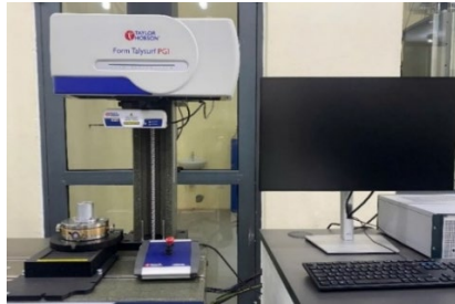
Fig. 2. Form Talysurf measuring machine
