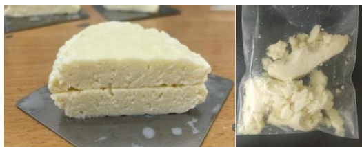
Fig 3. The structure of cheese reference cheese before and after being subjected to the force of the texture probe
