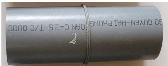
Fig. 3. Welding specimen of PVC-U 75 mm pipe
