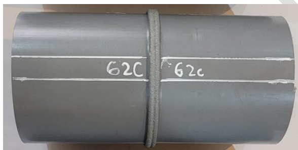
Fig. 4. Welding specimen of PVC-U 110 mm pipe
