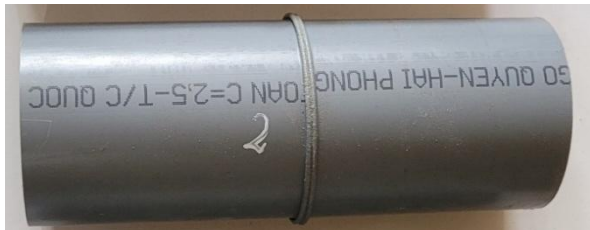
Fig. 3. Welding specimen of PVC-U 75 mm pipe
