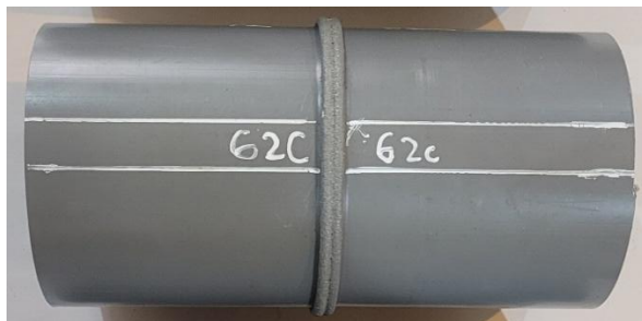
Fig. 4. Welding specimen of PVC-U 110 mm pipe
