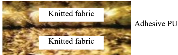
Fig. 2. Structure of waterproof fabric for L3 layer
