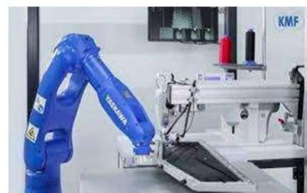
Fig. 2. Robotic arm for garment assembly
