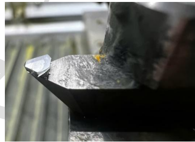
Fig. 5. Cutting tool model NN60R0635mWGC-MS0454
