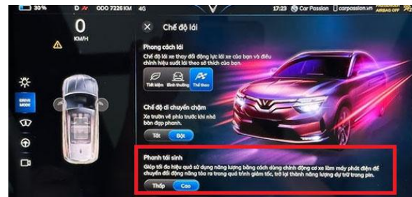
Fig. 6. Two regenerative braking modes of VinFast VF8
