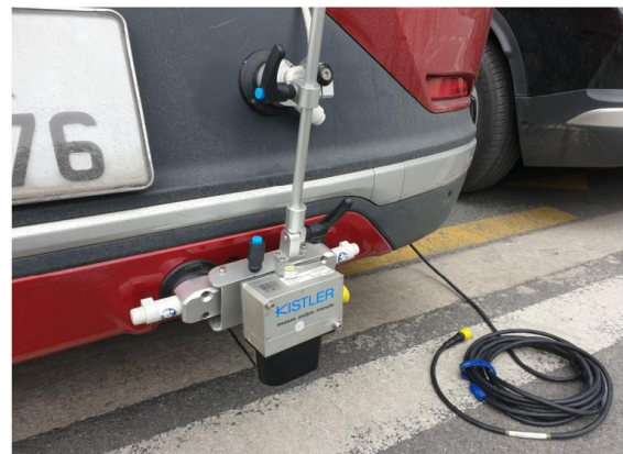
Fig. 9. The installation of S-Motion sensor
