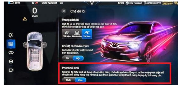
Fig. 6. Two regenerative braking modes of VinFast VF8
