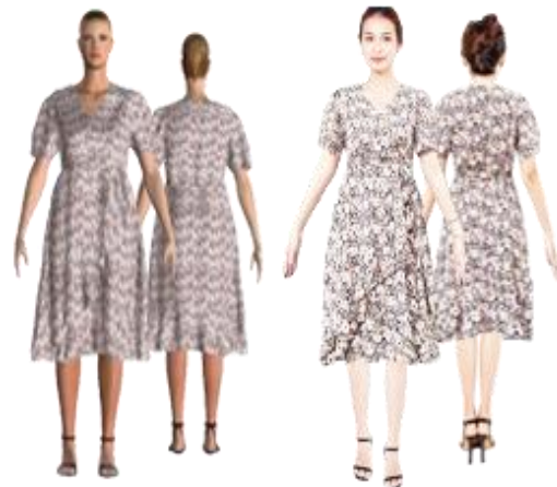
a) 3D Simulation b) Actual product after sewing Fig. 12. Visual comparison between 3D simulation and actual product after sewing.
