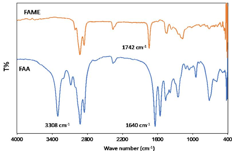
Fig. 3. FTIR spectra of fatty acid amide (FAA) and fatty acid methyl ester (FAME)
