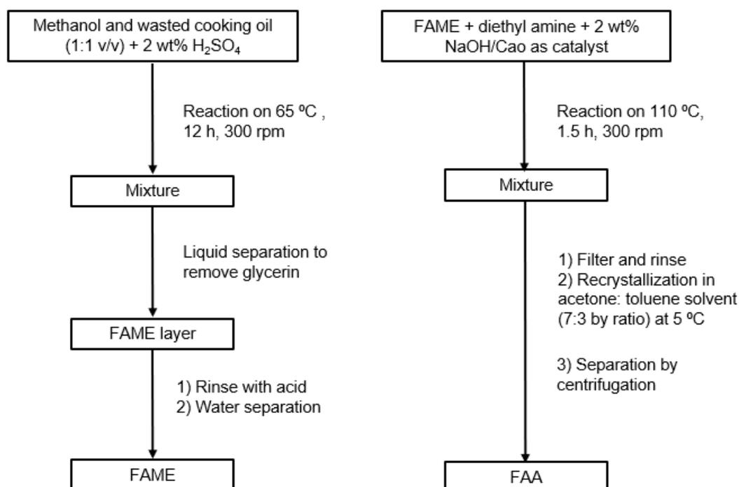
Fig. 1. Synthesis procedure of FAA from waste cooking oil
