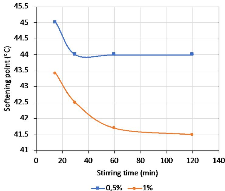
Fig. 7. Effect of stirring times to softening point
