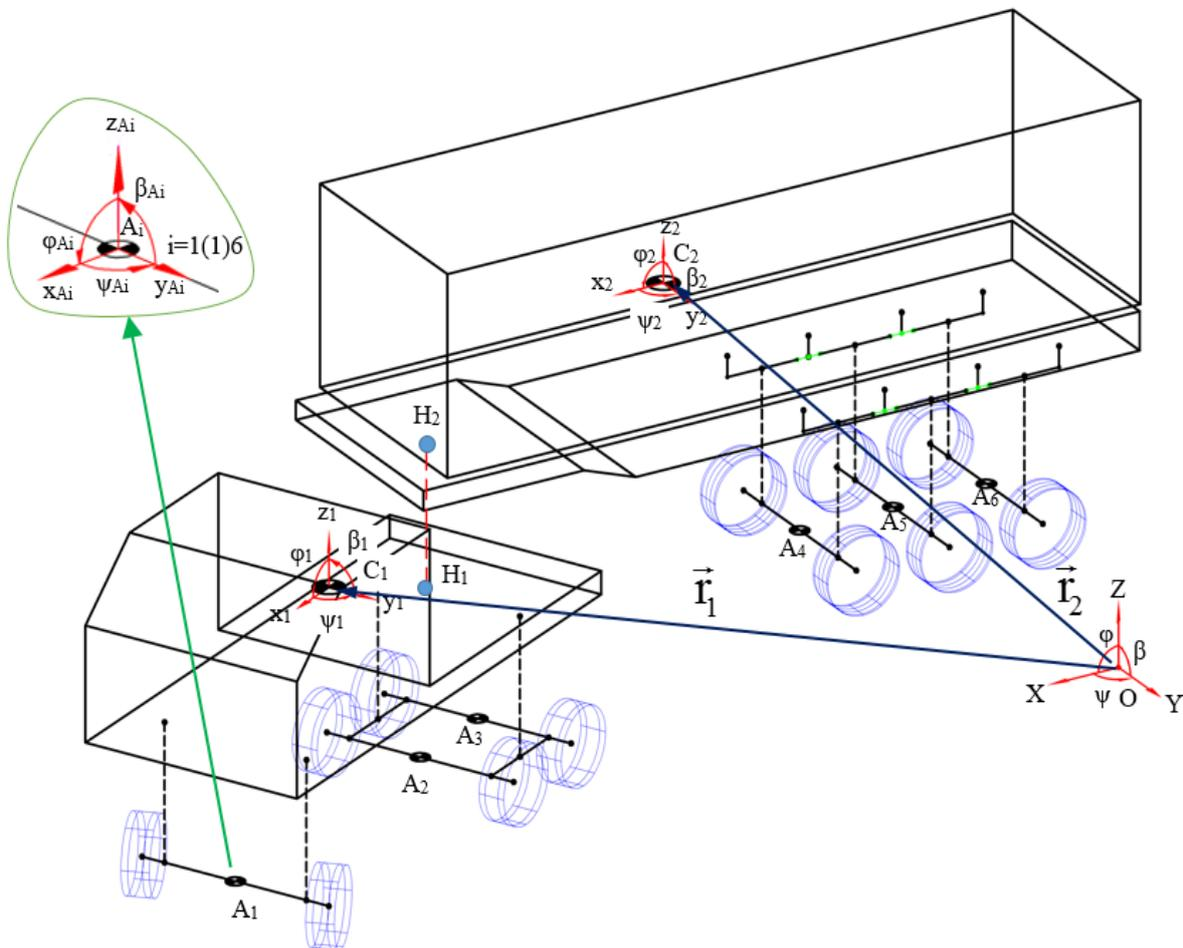
Fig. 2. Tractor semitrailer vehicle coordinate systems
