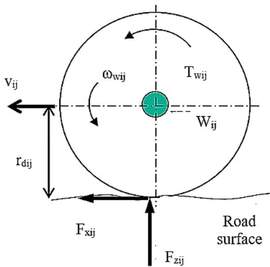
Fig. 4. Schematic of wheel dynamics
