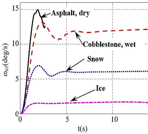
Fig. 10. Yaw rate of sprung mass of semitrailer
