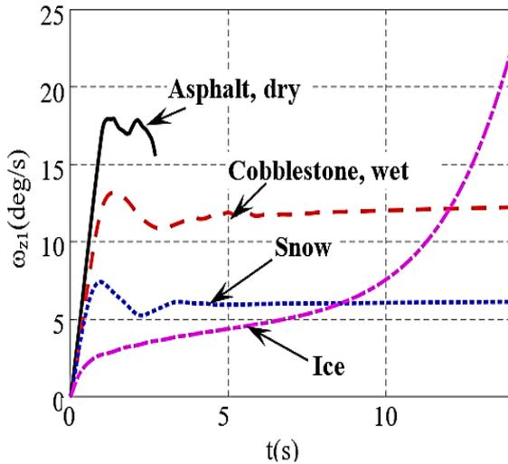
Fig. 9. Yaw rate of sprung mass of tractor
