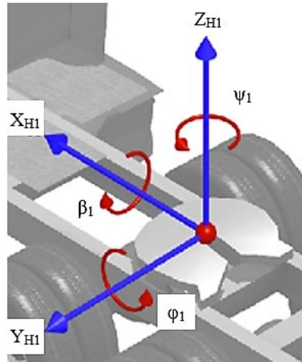
Fig. 5. Model of fifth wheel hitch
