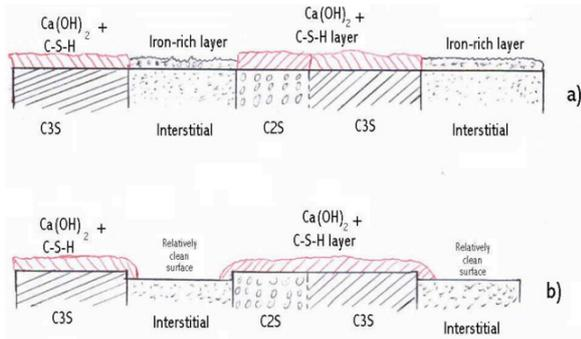
Fig. 6. Hydration process of cement with (b) and without additives TIPA (a)
