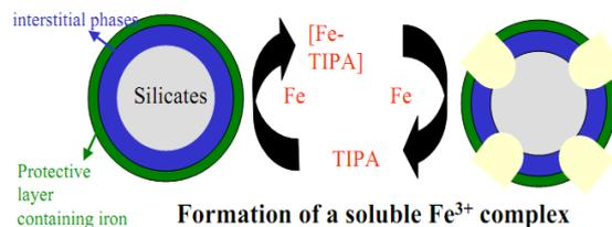
Fig. 3. Schema displaying the influence of TIPA with ferrite, proposed by Gartner and Myers
