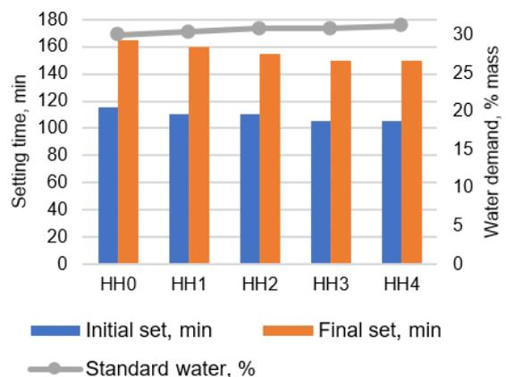
Fig. 10. The consistency and the setting time of cement
