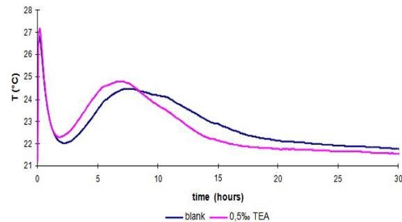
Fig. 2. Heat of hydration
