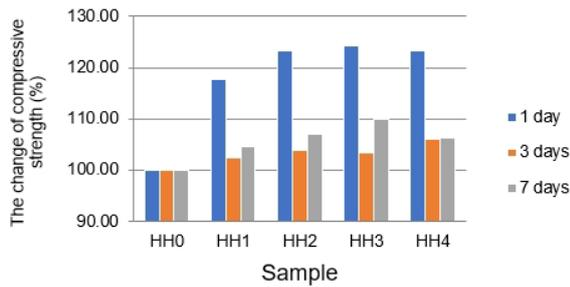
According to the results in Table 9, Table 10 and Fig. 11, the compressive strength at the age of 1 day, 3 days and 7 days increased. The compressive strength at the age of 1 day (sample HH3 with 0.01% TIPA + 0.02% TEA) is the highest with an increase of 24.21%. The flexural strength and compressive strength of the mixed admixture samples (containing TIPA + TEA) are higher than that of the single admixture sample HH1 (0.02% TEA).
