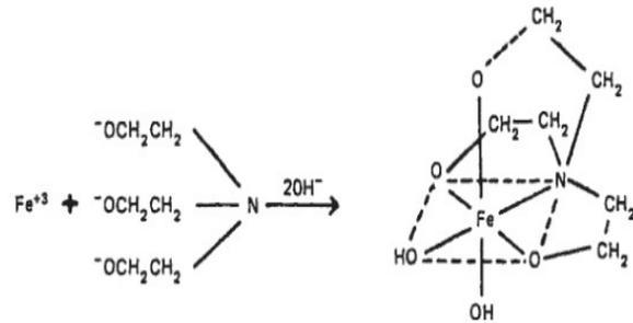
Fig. 1. Solubilization of the ferric ion in Portland Cement by TEA
