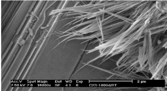
Fig. 1. The production CSH of the  $C_2S$  - hydration in cement.
