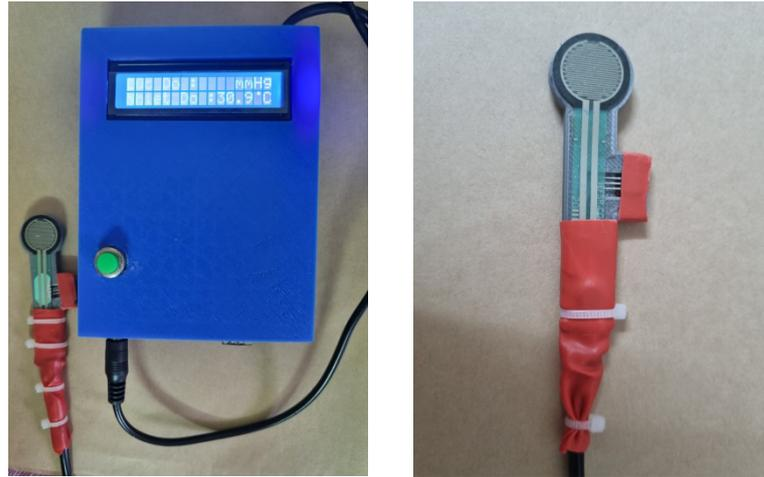
Fig. 3. Force Sensing Resistor (Length 6cm, Overall width 1.9cm, sensor area diameter 1.27cm)
