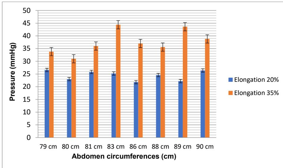
Fig. 5. The graph of mean pressures of the 8 abdomen circumferences measured by the sensor with elongation of 20% and 35%.
