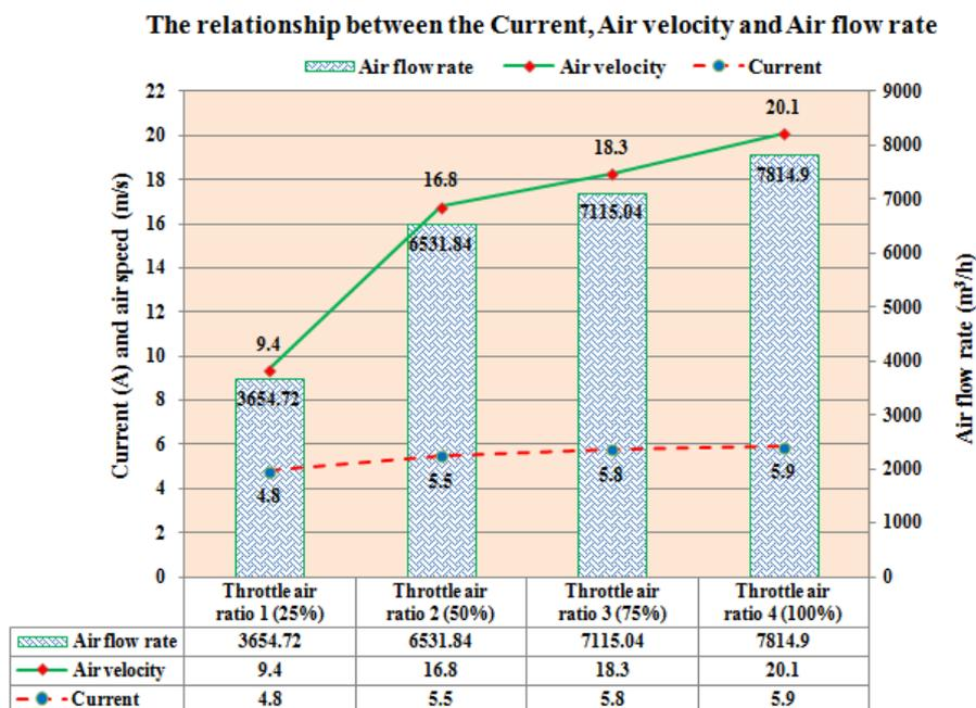
Fig. 4. Graph showing the relationship between air velocity and air flow when testing with drying fan
