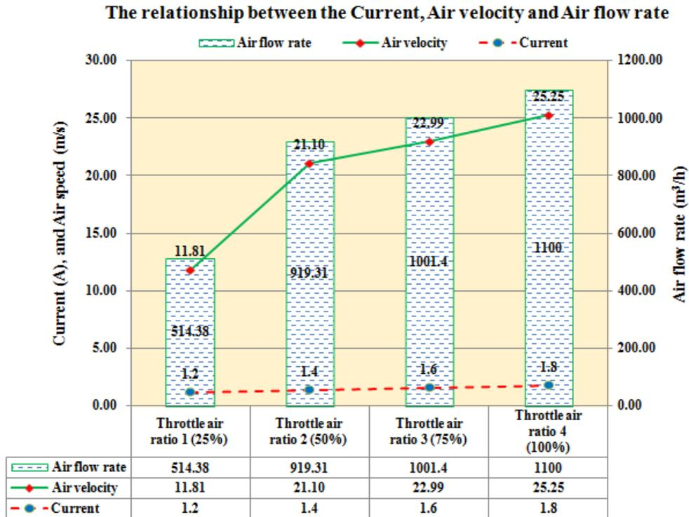
Fig. 5. Graph showing the relationship between air velocity and air flow when testing with furnace fan
