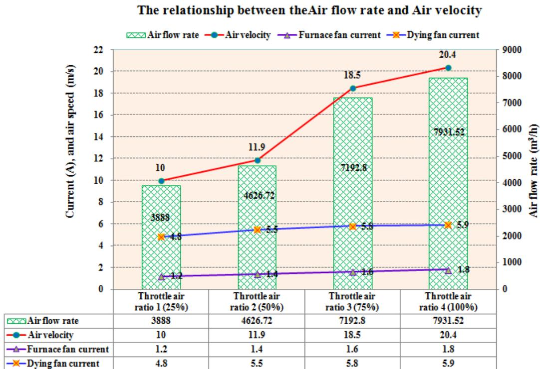
Fig. 6. Graph showing the relationship between air velocity and air flow when testing using furnace fan and drying fan
