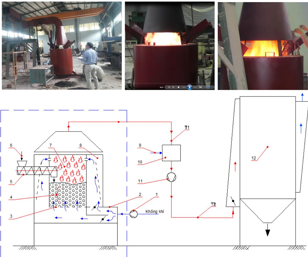
Fig. 3. Schematic diagram of the experimental furnace. 1- Furnace fan; 2- Co-Combustion and Gasification furnace; 3- Grate furnace; 4- Three zones: the combustion/oxidation zone, the pyrolysis zone and the reduction zone; 5- Screw conveyor; 6- Fuel; 7- Combustion of syngas; 8- Air chamber; 9- Air; 10- Mixing chamber; 11- Drying fan; 12- Drying system/Dryer; T1- Flame temperature; T2- Drying agent temperature.
