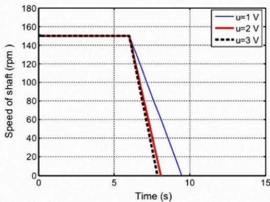
Fig 1. Comparing shaft deceleration time with different currents.
