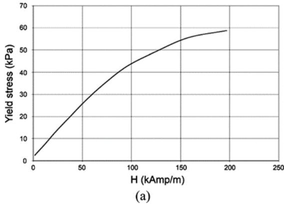
Fig. 3. Describe the effect of magnetic field on stress.
