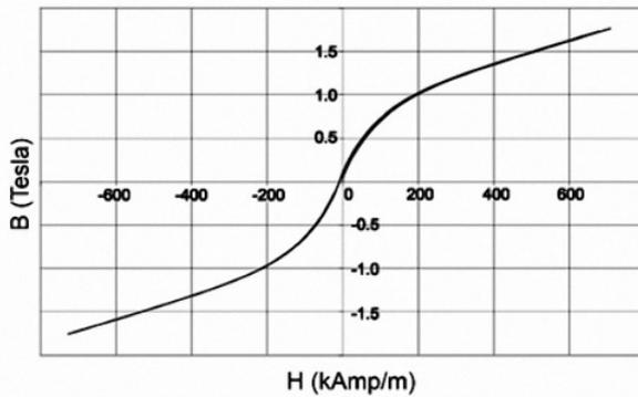
Fig. 4. Magnetic particle Saturation.
