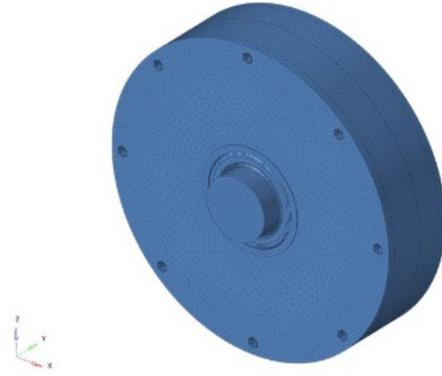
Fig. 9. Finite Element Model of MRB.
