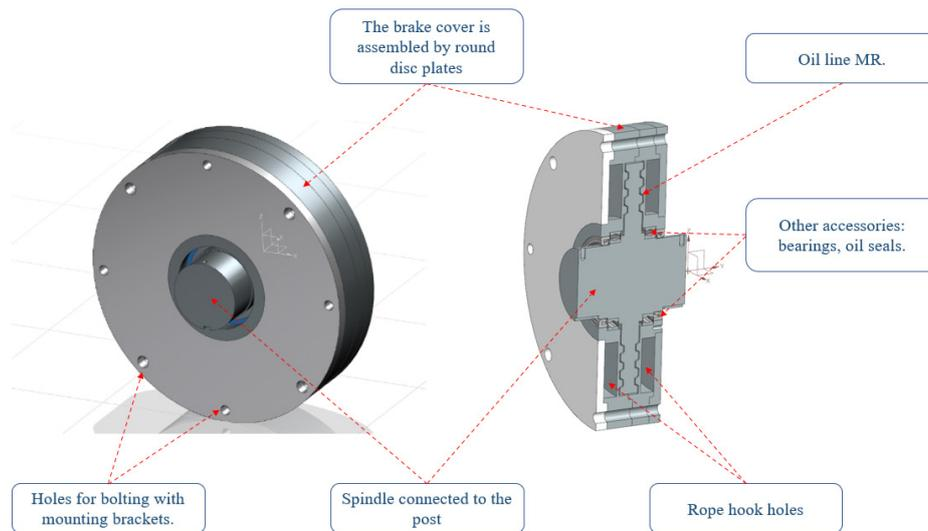
Fig. 6. Magnetic brake construction.
