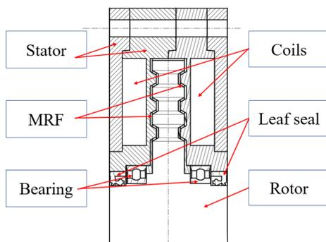
Fig. 7. Description of brake structure with MRF
