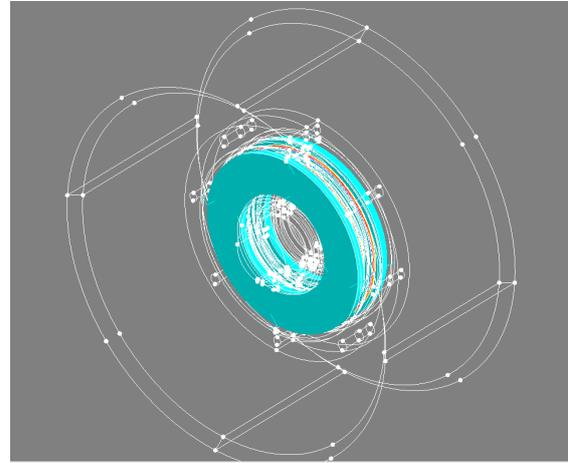
Fig. 10. Hollow (non-mesh) coil model.
