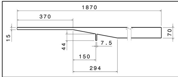
Fig. 3. 2D Geometry of the diffuser (Unit: mm)
