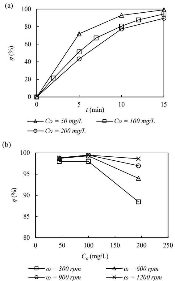
Fig. 4. The influence of the initial MB concentration on the MB treatment efficiency of the (a) conventional ozonation and (b) ozonation combined HP2R
