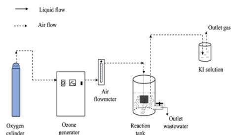
Fig. 1. Conventional ozonation experimental setup
