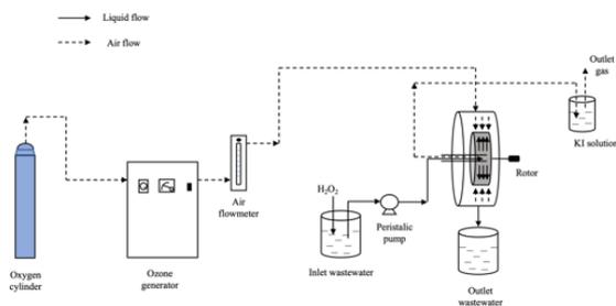
Fig. 2. Schematic diagram of the combined ozonation with HP2R experimental setup
