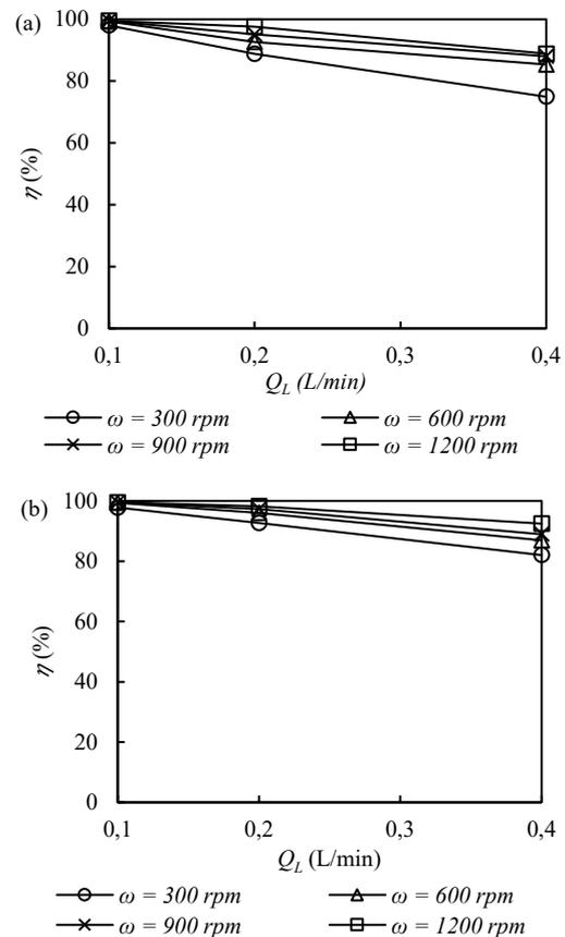
Fig. 6. Effect of  $Q_L$  on decolorization efficiency at (a)  $Q_G = 0.5$  L/min and (b)  $Q_G = 1$  L/min
