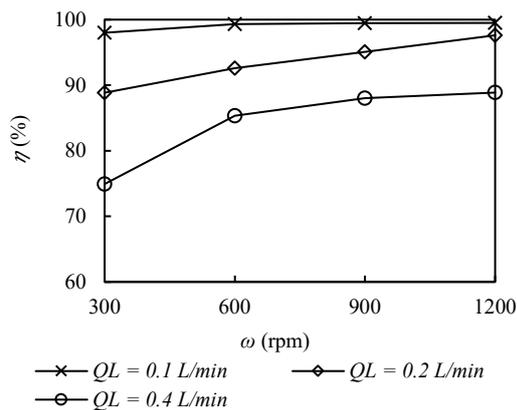
Fig. 5. Effect of rotor speed on decolorization efficiency
