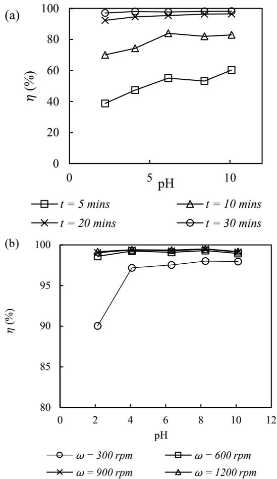
Fig. 3. Effect of pH on decolorization efficiency (a) conventional ozonation, (b) ozonation combine HP2R
