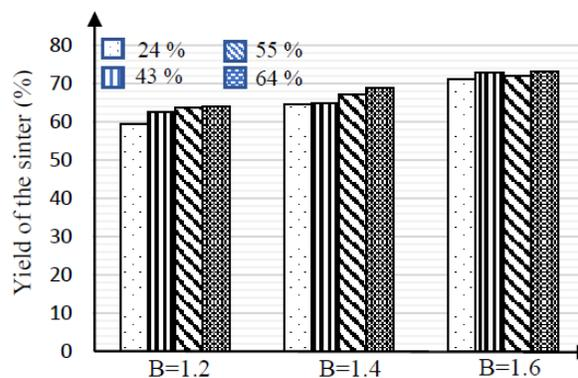
Fig. 2. Effect of basicity on yield of the sinter.
