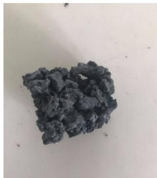
Fig. 5. Sinter sample after softening measurement at the temperature of 1200 °C.
