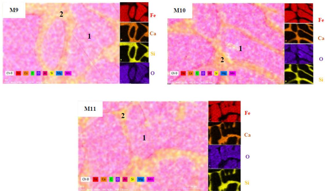
Fig. 8. Energy dispersive X-ray spectroscopy mapping results of the sinter.
