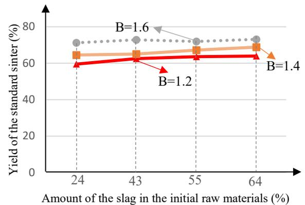
Fig. 3. Effect of slag amount on the strength of sinter.
