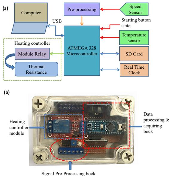
Fig. 3. The designation and schematic of the data acquisition module, (a)-the principle schematic, and (b)-the design of DAM
