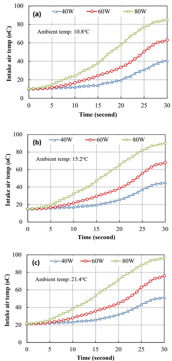
Fig. 5. Comparison of intake air temperature as a function of time at different ambient temperature conditions
