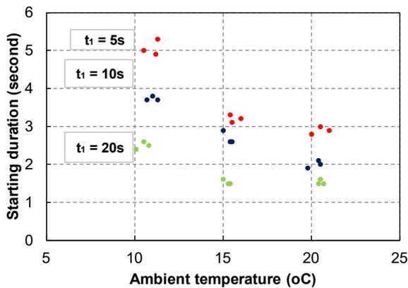
Fig. 6. Comparison of starting duration at different ambient temperature conditions
