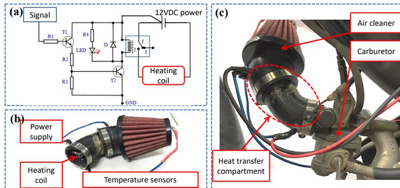
Fig. 2. The designation and schematic of the EHS : (a)-the principle of the heating controller module, (b)-the heating coil and heat transfer compartment, and (c)-the retrofitted intake manifold with EHS
