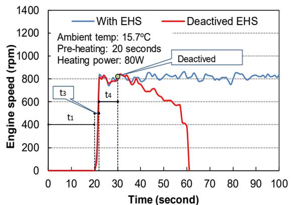
Fig. 7. Comparison of idling speed variation in the case of continuous using EHS and EHS deactivating at different ambient temperature conditions
