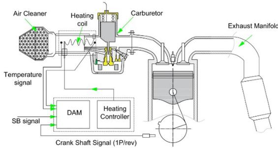
Fig. 1. The principle schematic of the EHS
