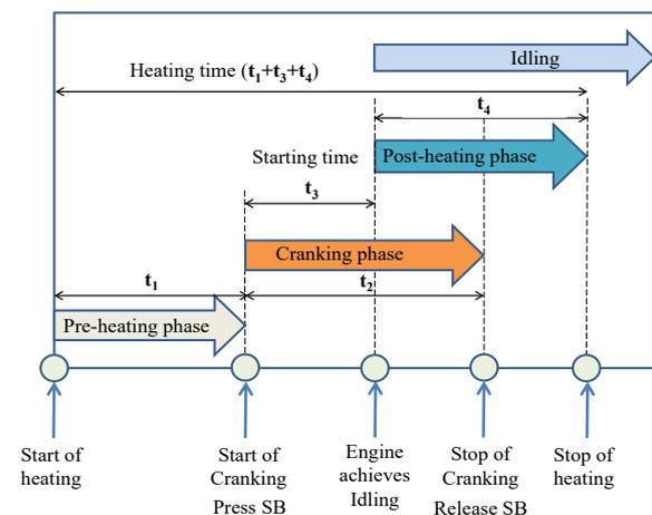
Fig. 4. The experimental procedure diagram
