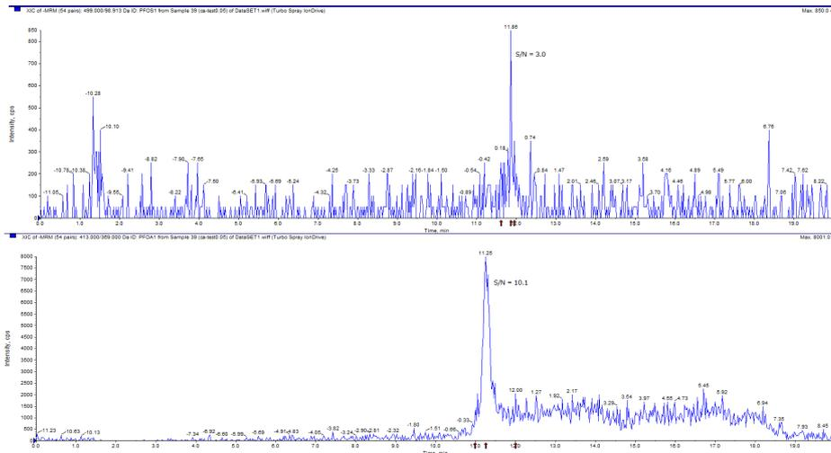
**Fig. 5. Signal-to-noise ratio of PFOS (upper) and PFOA (lower) at 0.05 ppb**
