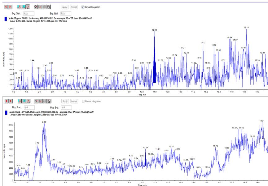
Fig. 2. Chromatograms of PFOS (upper) and PFOA (lower) with the conventional elution mode
