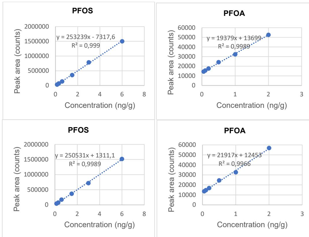
Fig. 6. Calibration curves, regression equations and coefficients of determination of PFOS and PFOA on the solvent (upper) and on the blank matrix (lower)
