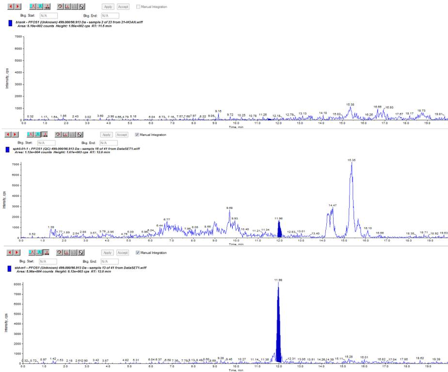
**Fig. 4. Chromatograms of blank samples, spiked samples, and standard solutions of PF**
