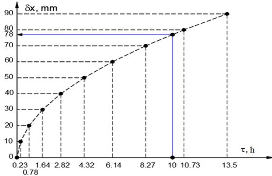
Fig. 4. Relationship  $\delta x = f(\tau)$  of freezing process on flat surface
