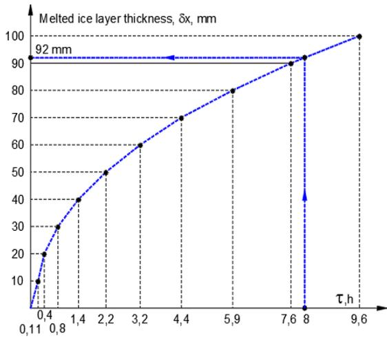
Fig. 6. Relationship  $\delta_x = f(\tau)$  of defrosting process on pipes
