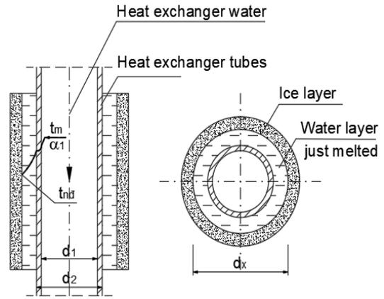
Fig. 5. Model of defrosting problem on pipe surface
