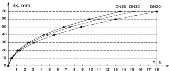
Fig. 2. Relationship  $\delta_x = f(\tau)$  of freezing process on steel pipe surface
