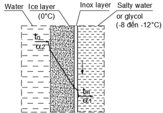
Fig. 3. Mathematical model of the freezing process on flat walls
