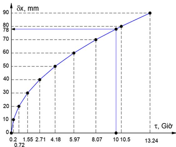
Fig. 8. Relationship between melting ice layer thickness and time,  $\delta_x = f(\tau)$
