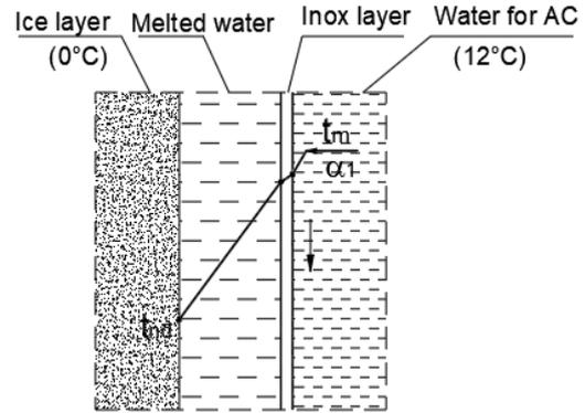
Fig. 7: Model of defrosting process on flat surface
