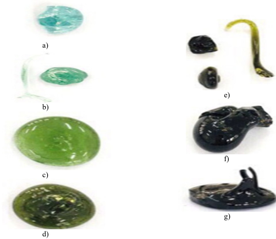
Fig. 1. Images of glass samples with different ratios of dust and glass (a) 0:100; (b) 0.5:99.5; (c) 1:99; (d) 2:98; (e) 5:95; (f) 10:90; (g) 15:85
