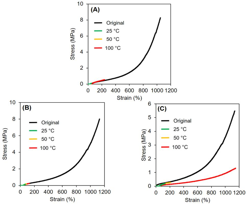
Fig. 4. Stress-strain curves of (A) NR/5ZnO/1.0S , (B) NR/3MgO/2ZnO/1.0S, and (C) NR/5MgO/1.0S before and after self-healing for 12 hours at 25 °C, 50 °C, and 100 °C
