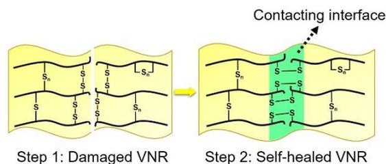
Fig. 8. Proposed mechanism for self-healing process of vulcanized natural rubber
