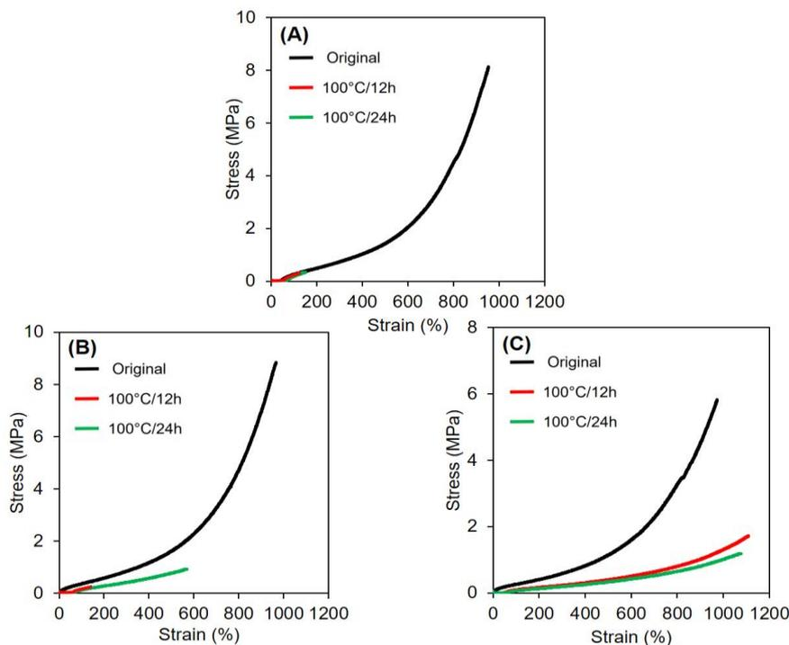
Fig. 7. Stress-strain curves of (A) NR/5ZnO/1.5S, (B) NR/3MgO/2ZnO/1.5S, and (C) NR/5MgO/1.5S before and after self-healing process at 100 °C for 12 hours and 24 hours
