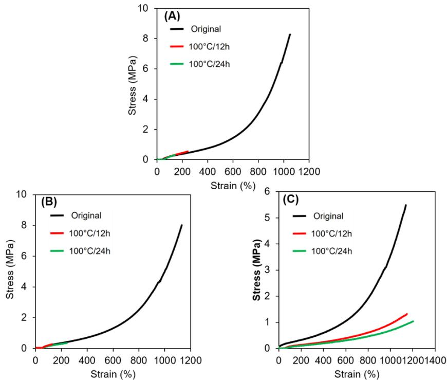
Fig. 6. Stress-strain curves of (A) NR/5ZnO/1.0S, (B) NR/3MgO/2ZnO/1.0S, and (C) NR/5MgO/1.0S before and after self-healing process at 100 °C for 12 hours and 24 hours
