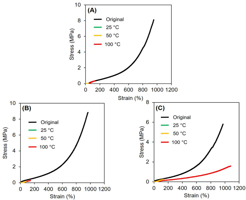
Fig. 5. Stress-strain curves of (A) NR/5ZnO/1.5S, (B) NR/3MgO/2ZnO/1.5S, and (C) NR/5MgO/1.5S before and after self-healing for 12 hours at 25 °C, 50 °C, and 100 °C
