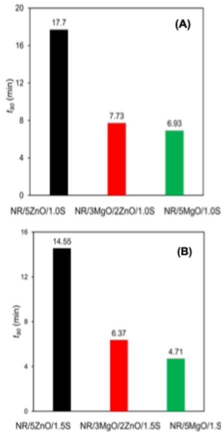
Fig. 2. Optimal cure time for V-NR prepared with 5ZnO, 3MgO/2ZnO, and 5MgO at sulfur content of (A) 1.0 phr and (B) 1.5 phr
