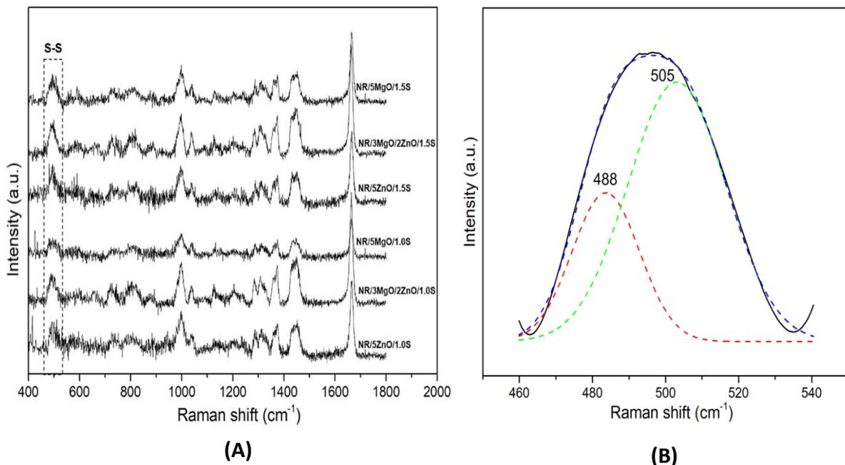
Fig. 3. Raman spectra for (A) V-NR and (B) its deconvolution
