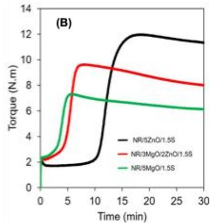
Fig. 1. Cure curves for V-NR samples prepared with 5ZnO, 3MgO/2ZnO, and 5MgO at sulfur content of (A) 1.0 phr and (B) 1.5 phr
