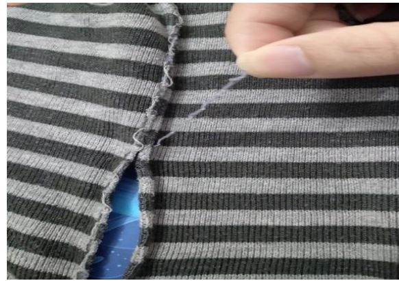
Fig. 2. Unraveling the linking stitches to get panels
