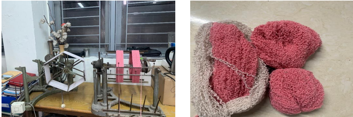
Fig. 4. Yarn reeling equipment and the ball of collected yarn
