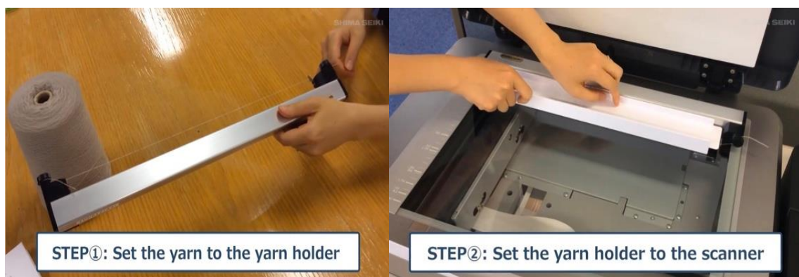
Fig. 5. Scanning the collected yarn
