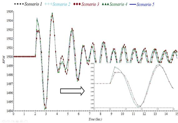
Fig. 7. Generator speed of conventional generator nearby in case 1.
