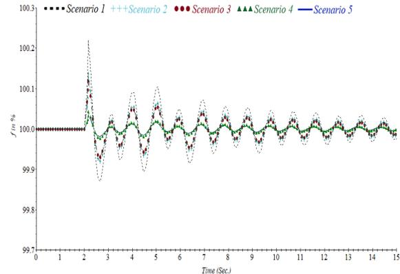
Fig. 6. The frequency response of the grid in case 1.
