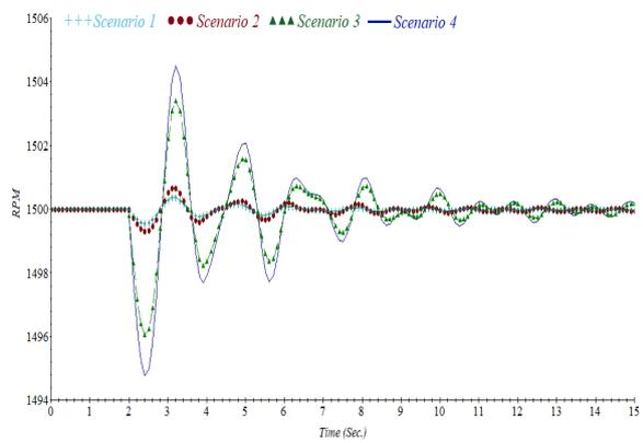
Fig. 11. Generator speed of conventional generator nearby in case 2.
