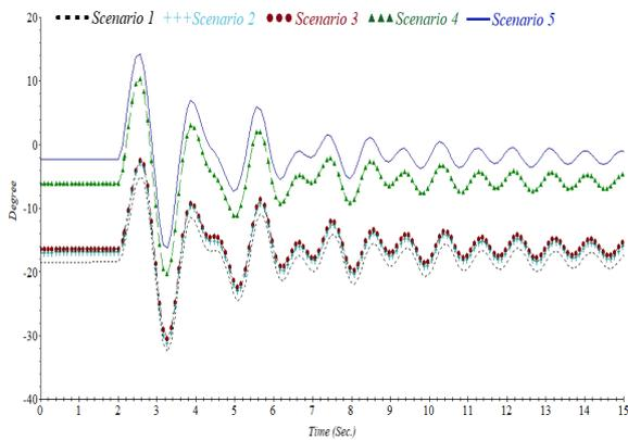
Fig. 8. Rotor angle of conventional generator nearby in case 1
