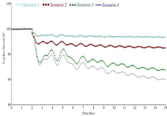
Fig. 9. The voltage response of the grid in case 2.
