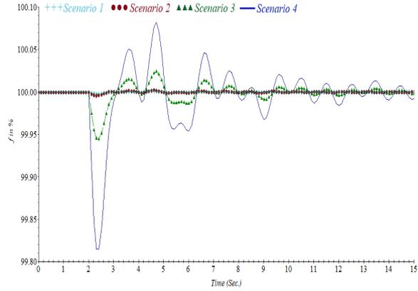
Fig. 10. The frequency response of the grid in case 2
