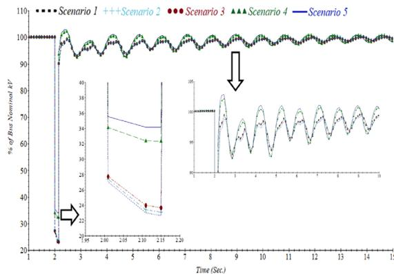
Fig. 5. The voltage response of the grid in case 1.
