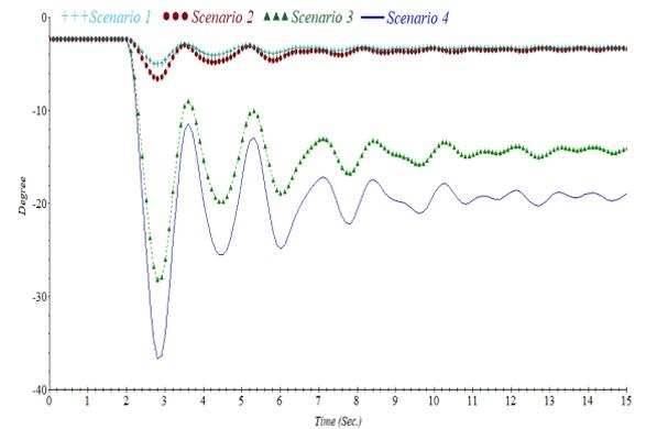
Fig. 12. Rotor angle of conventional generator nearby in case 2.
