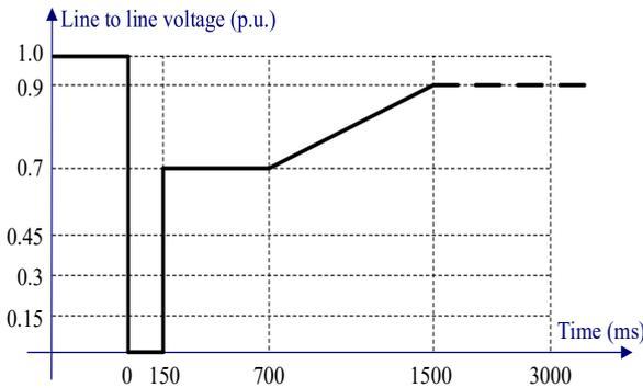
Fig. 4. The low voltage ride-through of grid code.
