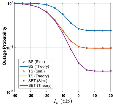
Fig. 2. Effect of  $I_p$  on the system outage probability with  $P_{PB} = 1$  dB.
