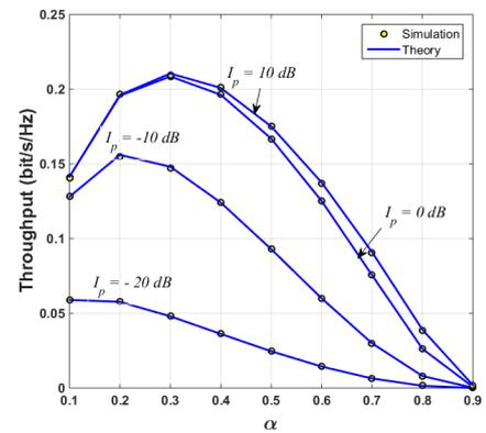
Fig. 5. Effect of  $\alpha$  on the system throughput in SBT scheme with different values of  $I_p$
