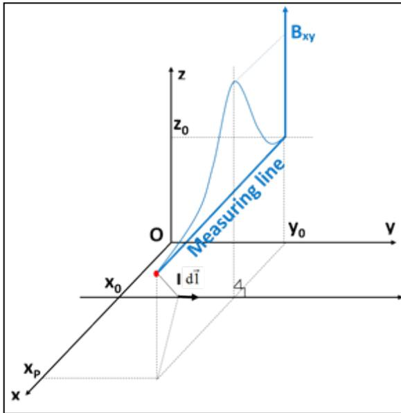
Fig. 1. A straight, infinite wire carrying a current I.
