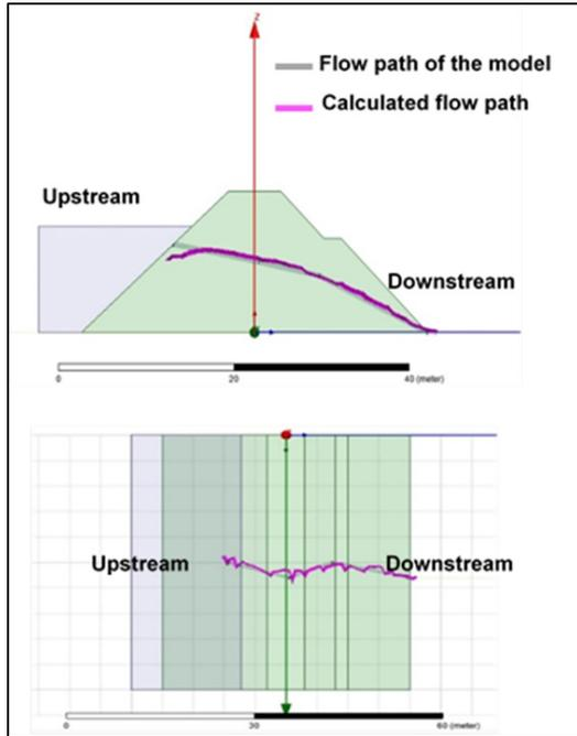
Fig. 3. The calculated preferential flow path of the hypothetical model.
