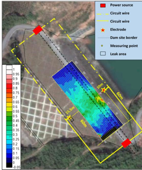
Fig. 6. The horizontal magnetic field of the study dam.
