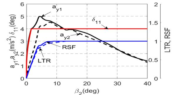
Fig. 8. Roll performance signature of a tractor semitrailer vehicle in  $\delta_{11stab}=4$ deg.
