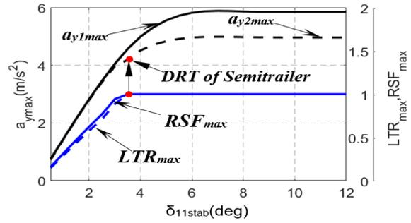
Fig. 9. Effect of road wheel steering angle on rollover condition of tractor semitrailer.
