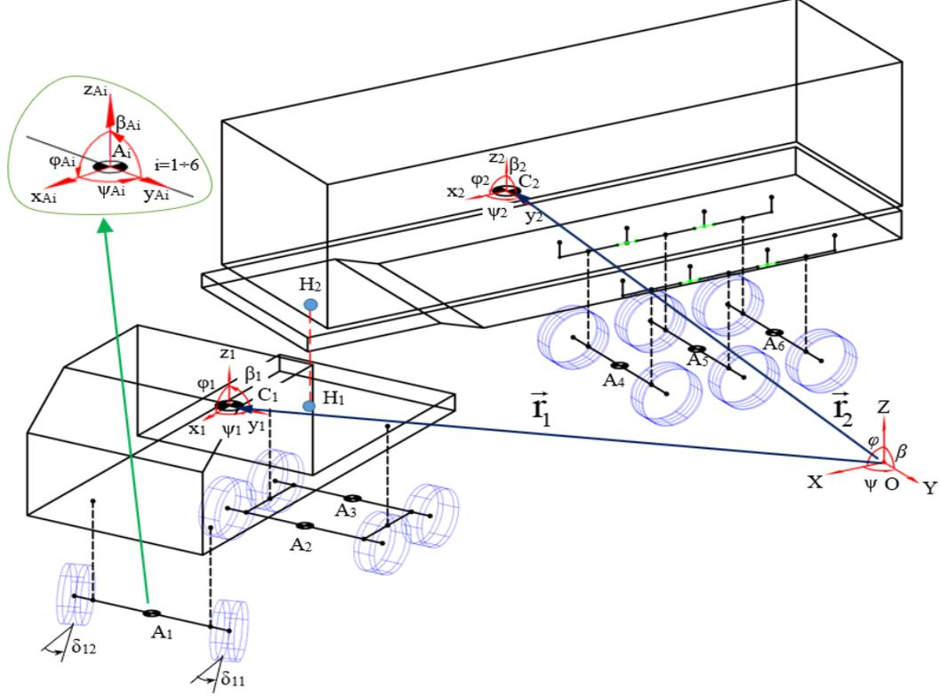
Fig. 2. Tractor-Semitrailer Coordinate Systems
