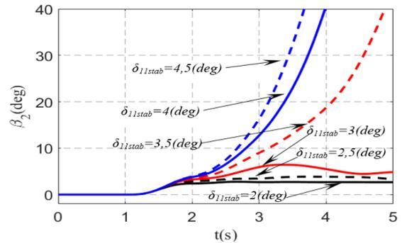
**Fig. 6.** Roll angle of the sprung mass of the semitrailer vehicle.
