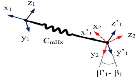
Fig. 4. Representation of the conventional fifth wheel hitch connection.
