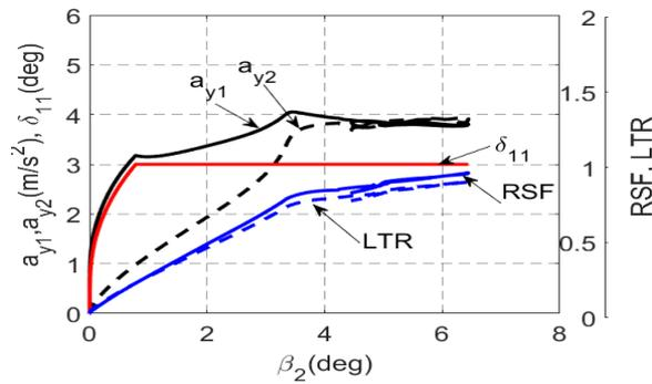
Fig. 7. Roll performance signature of a tractor semitrailer vehicle in  $\delta_{11stab}=3$ deg.
