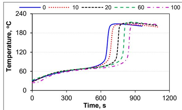
**Fig. 4.** The effect of the nano-silver content on the heat of curing reaction
