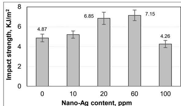
Fig. 7. The effect of the nano-silver content on the impact strength of composite
