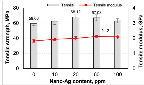
Fig. 6. The effect of the nano-silver content on the tensile properties of composite
