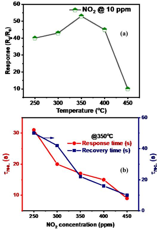
**Fig.8.** (a) Gas response and (b) response-recovery time at different temperatures.
