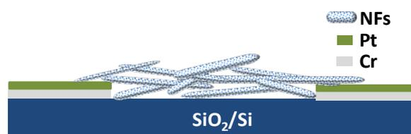
Fig.1. The scheme of a typical resistive sensor system.
