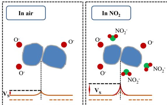
**Fig.7.** Schematic illustration the  $\text{NO}_2$  sensing mechanism of the  $\text{SnO}_2$  NFs.
