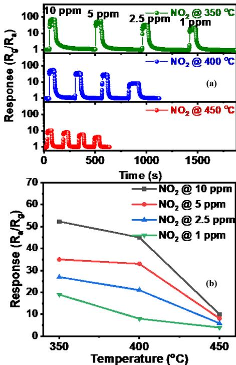
Fig. 5. (a) NO<sub>2</sub> sensing transients of the SnO<sub>2</sub> NFs at various operating temperatures and (b) Gas responses as a function of the NO<sub>2</sub> concentration at different temperatures.
