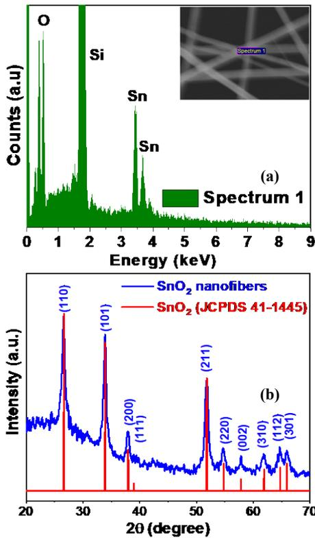
Fig 4. (a) The EDX spectrum and (b) XRD pattern of the SnO<sub>2</sub> NFs.
