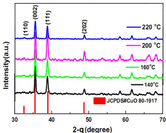
Fig.3. X-ray diffraction pattern of CuO nanoplates obtained by hydrothermal synthesis at different temperatures.
