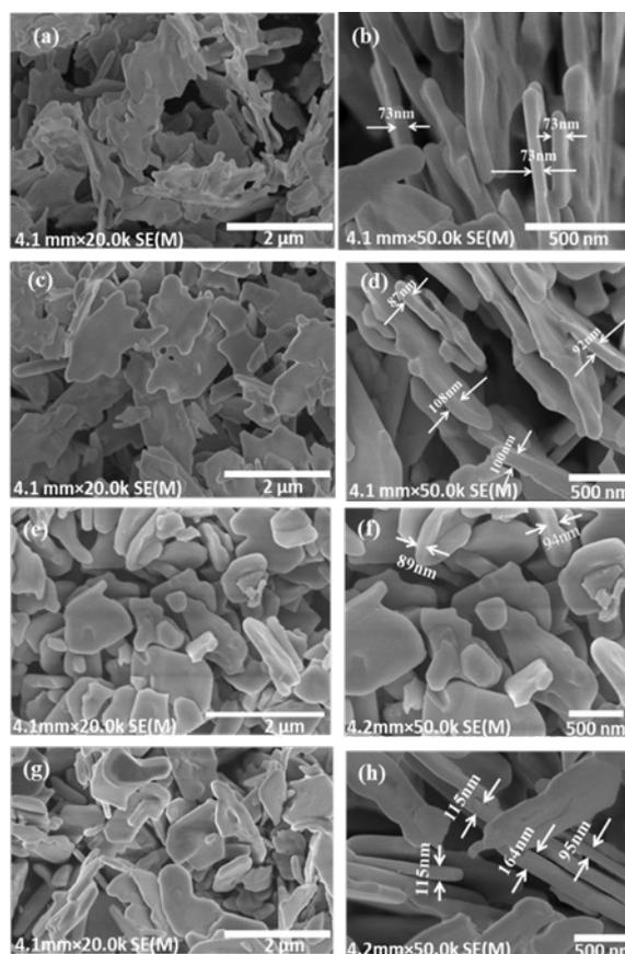
**Fig. 2.** FE-SEM images of CuO nanoplates with different hydrothermal temperatures: (a, b) at 140°C; (c, d) at 160°C; (e, f) at 200°C; (g, h) at 220°C.
