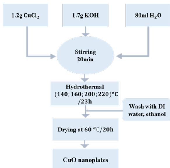
**Fig. 1.** Process of the hydrothermal synthesis of CuO nanoplates.
