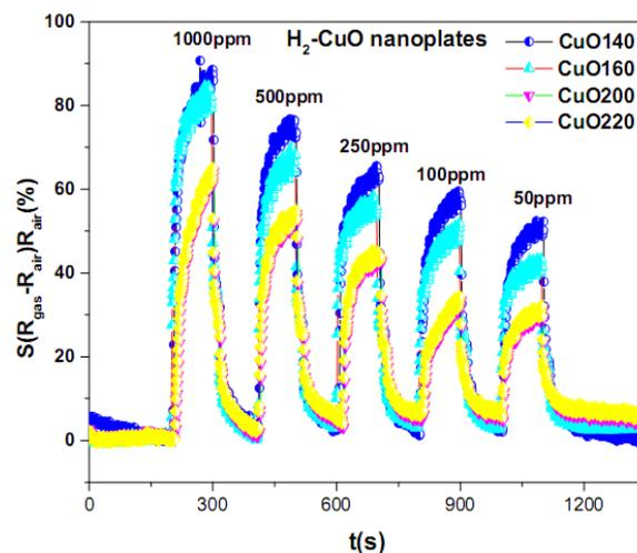
Fig.5. Comparative response result of the CuO nanoplates prepared at various hydrothermal temperatures to different  $H_2$  gas concentrations at the working temperature of 250°C.
