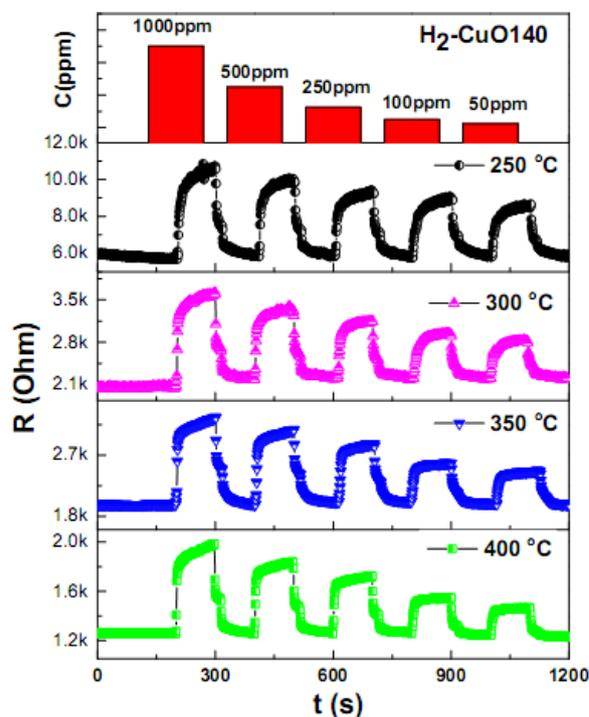
Fig.4.  $H_2$  sensing properties of the CuO140: transient resistance vs. time upon exposure to various concentrations of  $H_2$  at different working temperatures.
