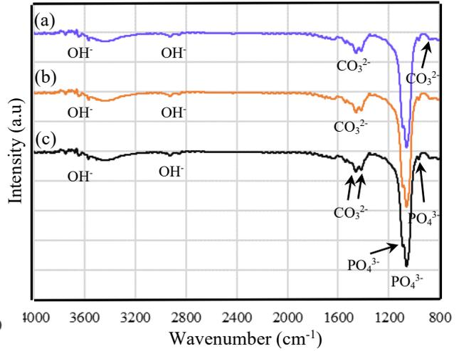
**Fig. 2.** FTIR pattern autoclaved HA samples at pH = 7÷8 (a); pH = 8÷9 (b) and pH = 9÷10 (c)
