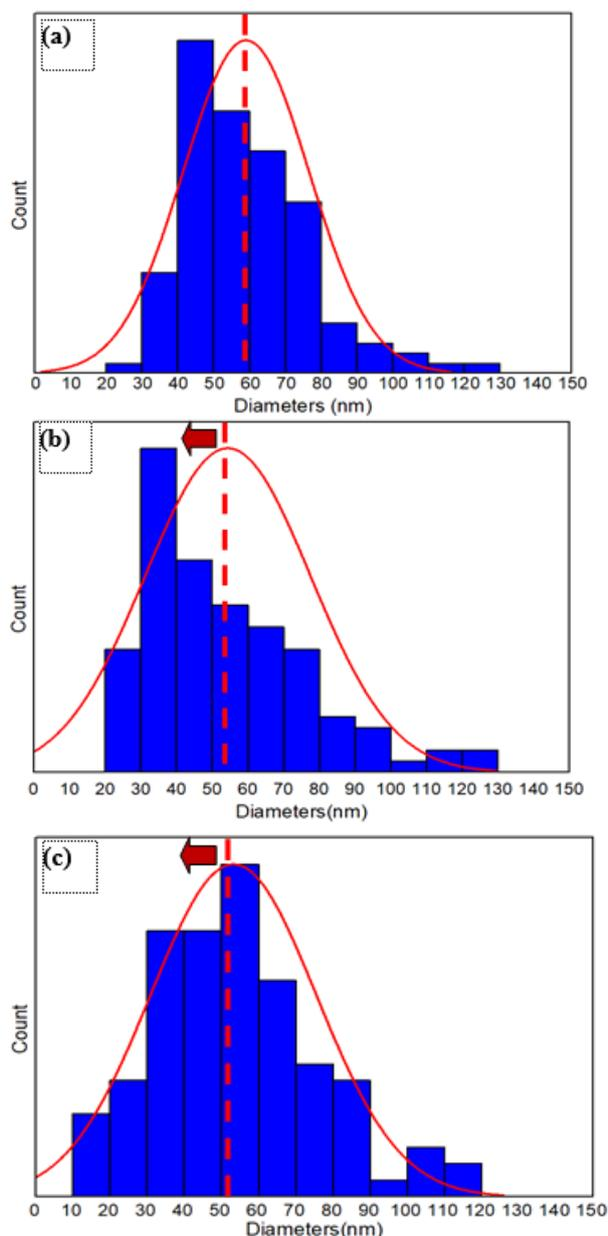
**Fig. 4.** Distributions of hydroxyapatite nanowire size with different pH values: (a) pH = 7÷8; (b) pH = 8÷9; (c) pH = 9÷10
