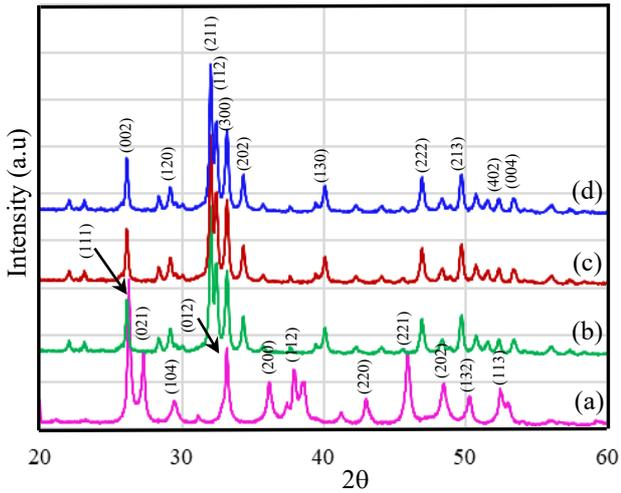
**Fig. 1.** XRD pattern of the raw clamshells (a) and HA powders autoclaved at different pH values: (b) pH = 7÷8; (c) pH = 8÷9; (d) pH = 9÷10
