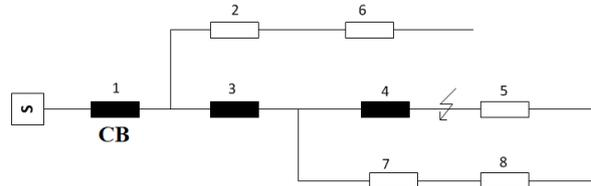
**Fig. 1.** Radial feeder using fault indicators
