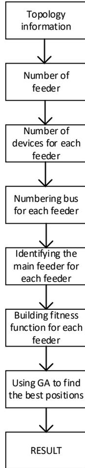
Fig. 3. The process of solving the problem
