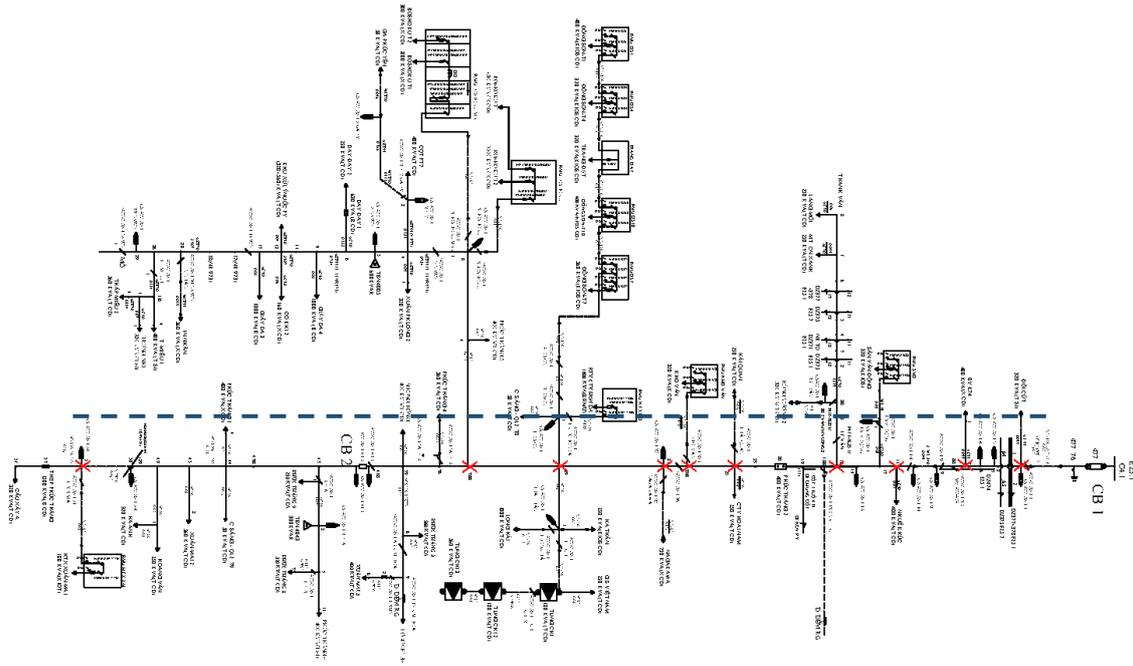
Fig. 5. Studied distribution network including main feeder (dash line) and final sectionalizers' placement (red X mark)
