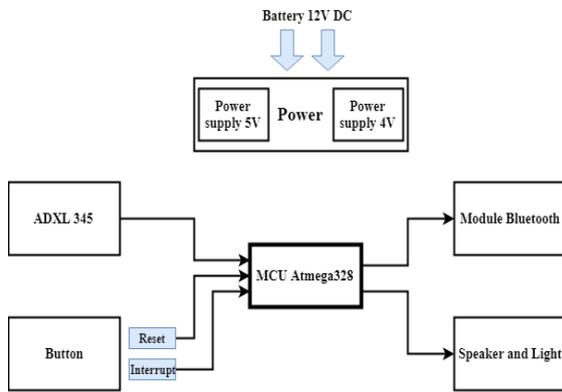
Fig. 3. Block diagram of motion sensor module
