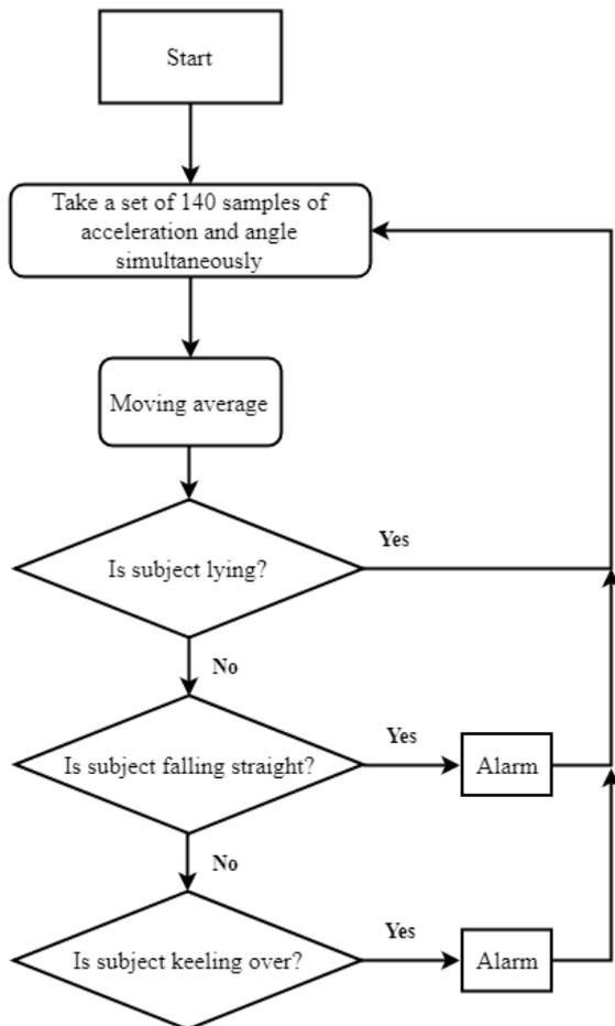
Fig. 1. Fall detection algorithm.
