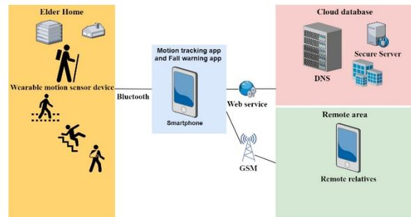
Fig. 2. Architecture of the proposed wireless fall warning system
