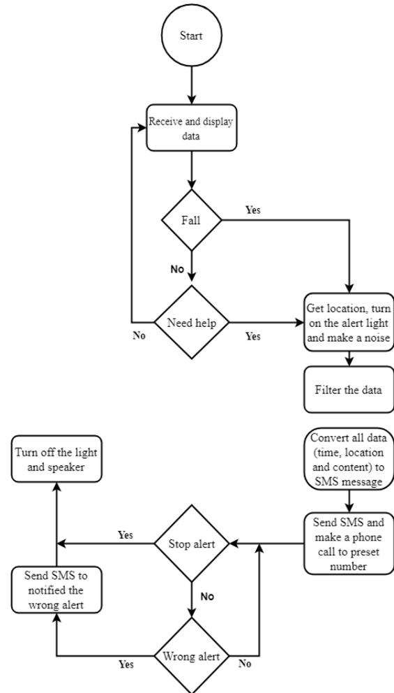
Fig 5. Alert mode diagram in Motion Tracking App
