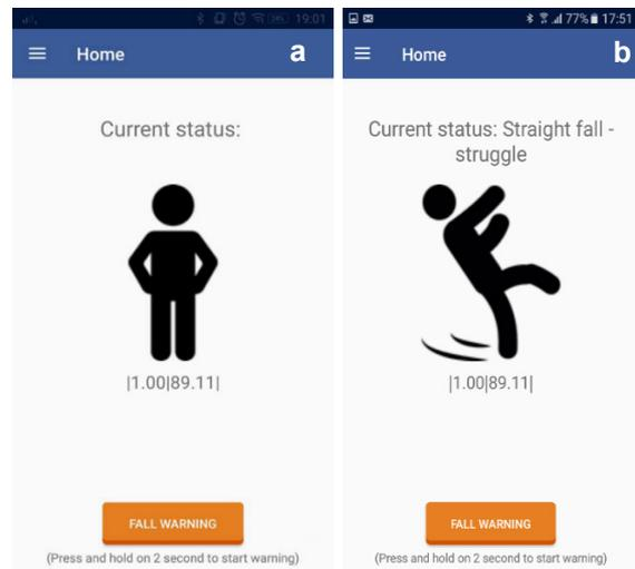
**Fig. 7.** a. Graphical interface of a smartphone shows status of person in Activities of Daily Living; b. Manual warning button and straight fall – struggle symbol when fall is detected.
