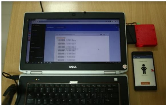
**Fig. 6.** The proposed system comprises motion sensor module (Redbox), fall warning application on smartphone and online data storage.
