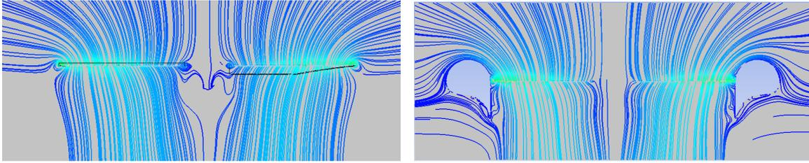
Fig. 10. Streamlines of free rotor (left) & shrouded rotor (right)
