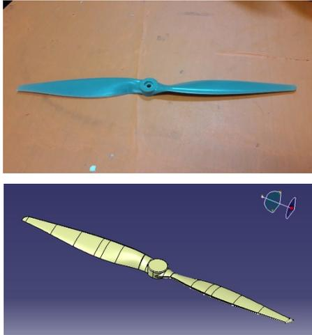
**Fig. 4.** APC propeller 15x4 & 15-inch rotor model
