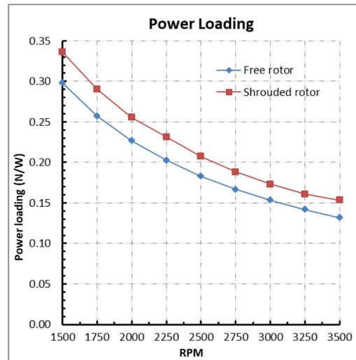
Fig. 9. Power loading of 9-inch rotor
