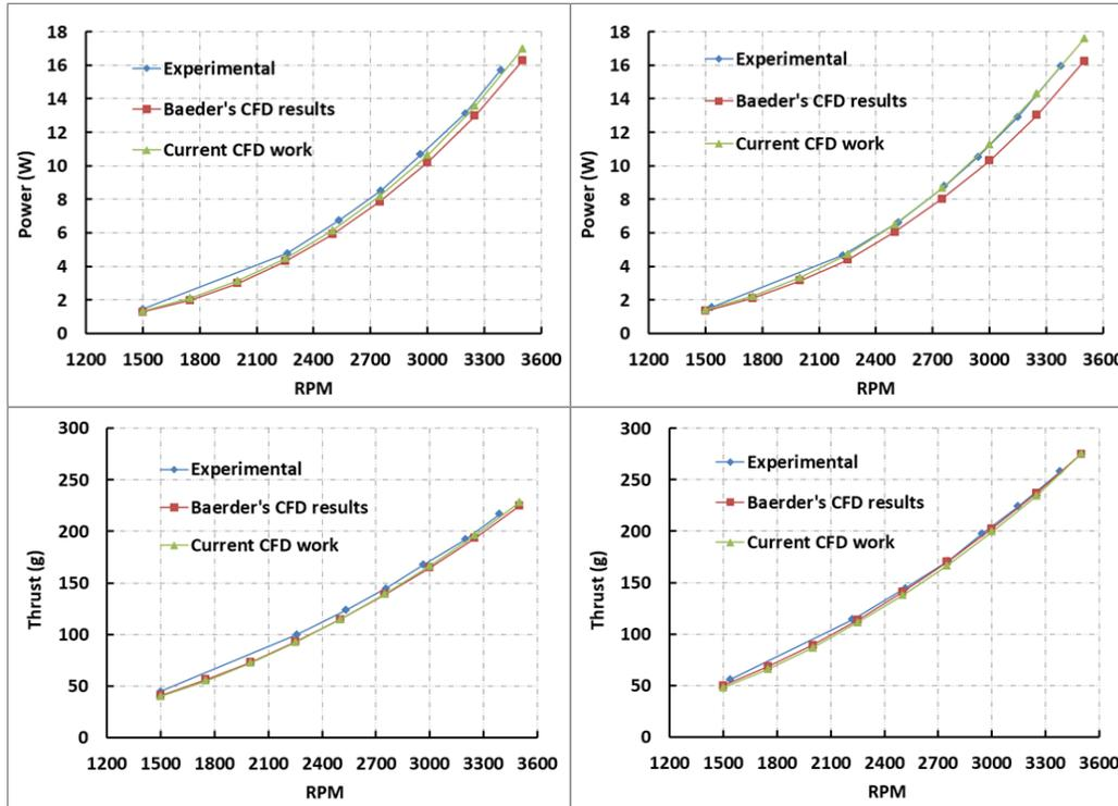
Fig. 11. CFD result comparisons: free rotor (left) & shrouded rotor (right)
