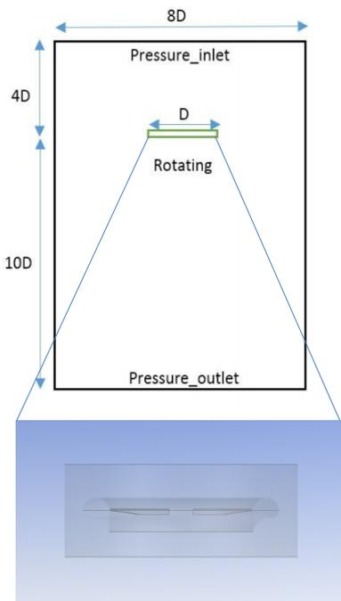
**Fig. 5.** Two flow domains & Rotating domain
