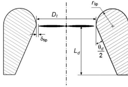
Fig. 2. Shroud design and its parameters
