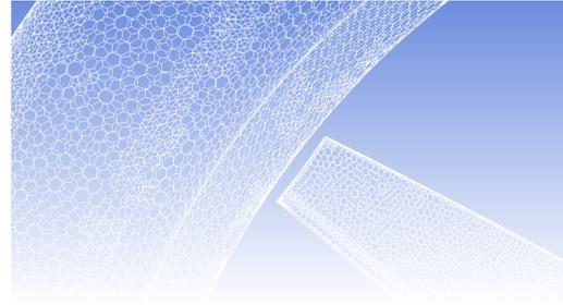
**Fig. 6.** Polyhedral mesh on blade and shroud surfaces
