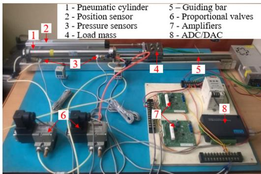
Fig. 2. Photo of the experimental test setup
