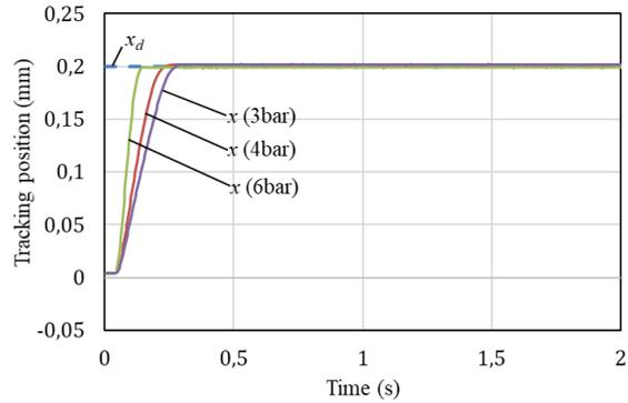
**Fig. 7** Tracking results with different source pressure (experiment)
