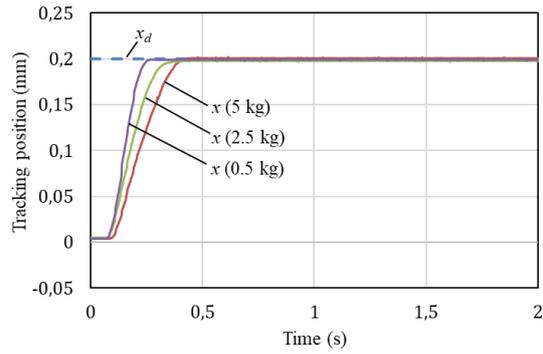
**Fig. 6** Tracking results with different external loads (experiment)
