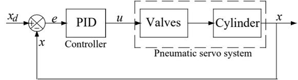
Fig. 3. Control diagram using PID controller
