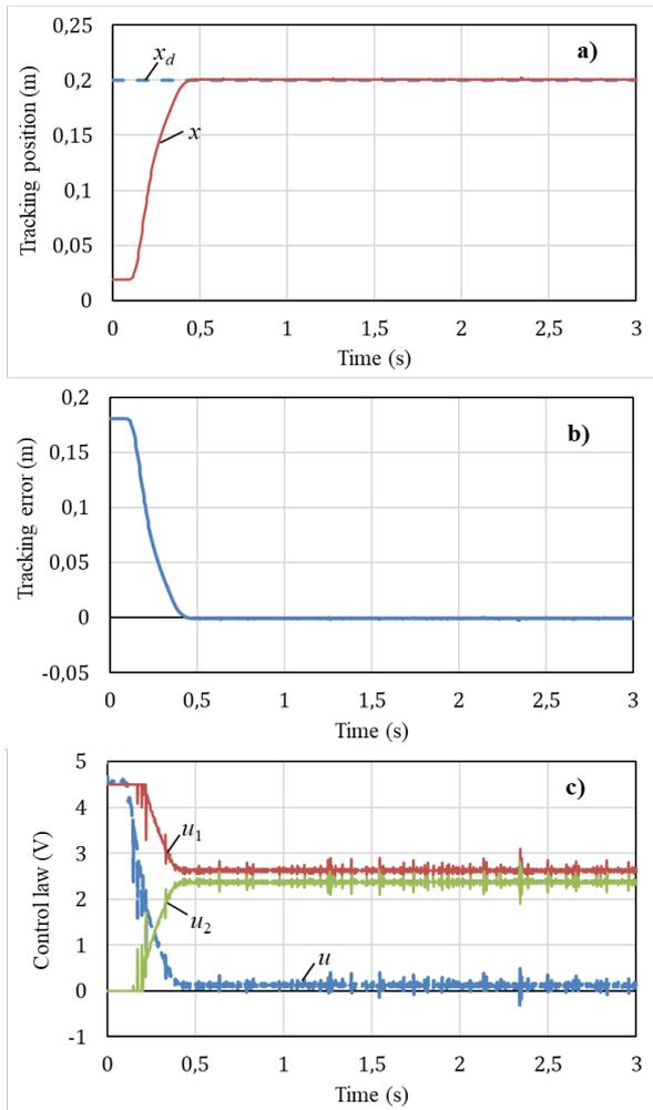
**Fig. 5.** Experimental result: a) tracking position, b) tracking error, c) control law (experiment)
