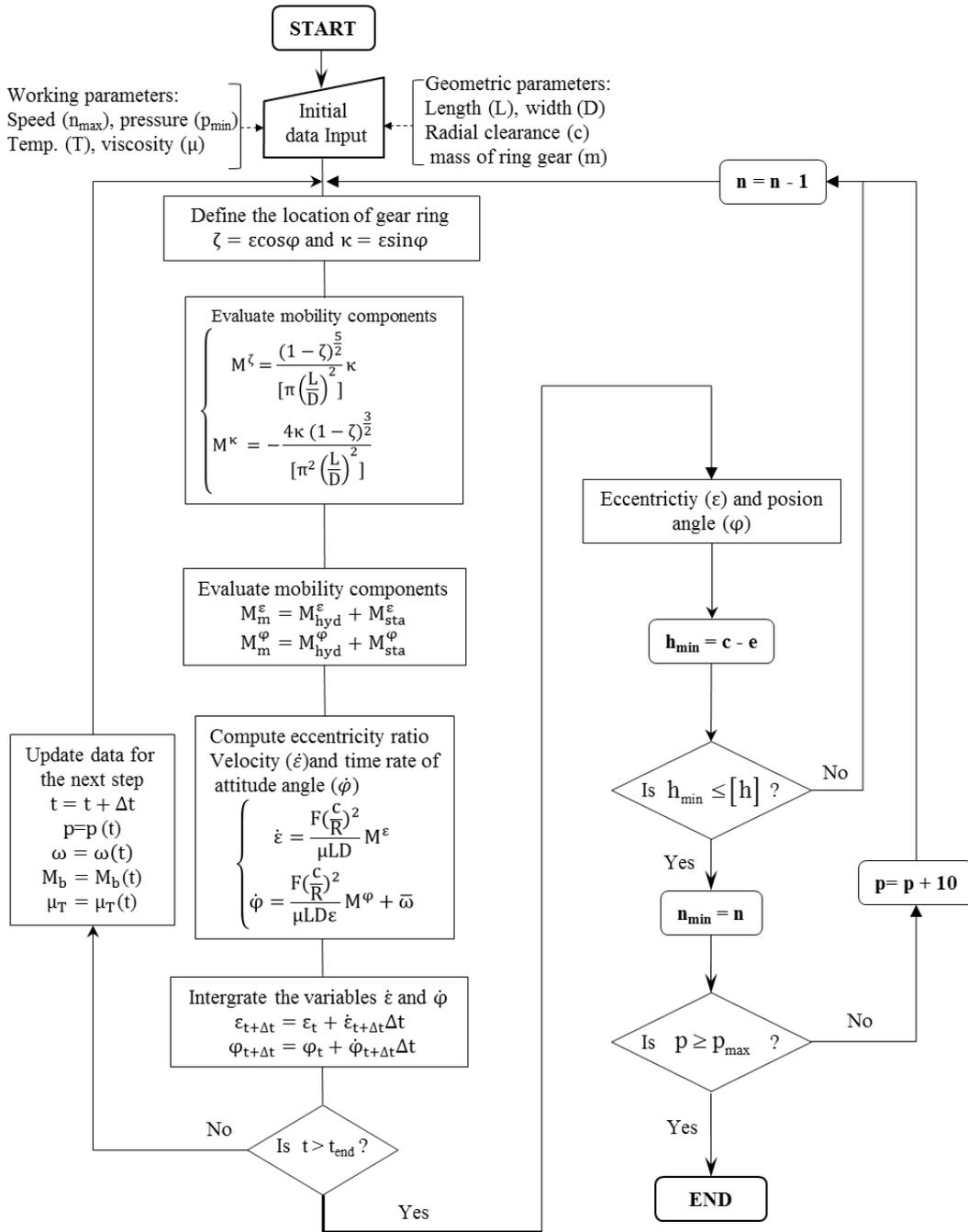
Fig. 3. Computational flow chart for calculation of minimum speed limit.
