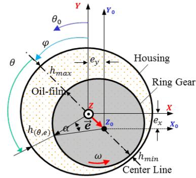
**Fig. 2.** Oil film thickness.
