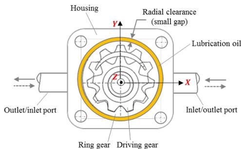
**Fig. 1.** Cross section of the internal gear motor.
