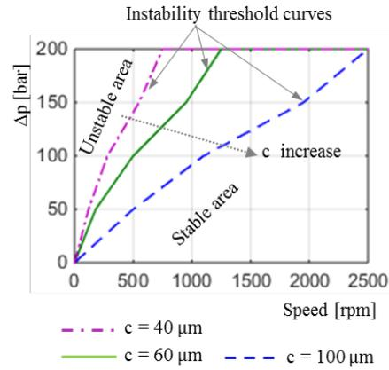
Fig. 5. Instability threshold for various values of the clearance.
