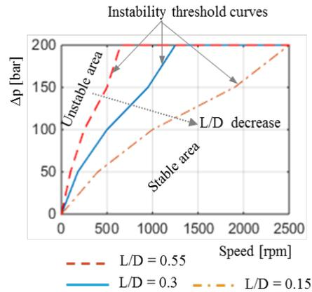
Fig. 6. Instability threshold for different values of  $L/D$  ratio.
