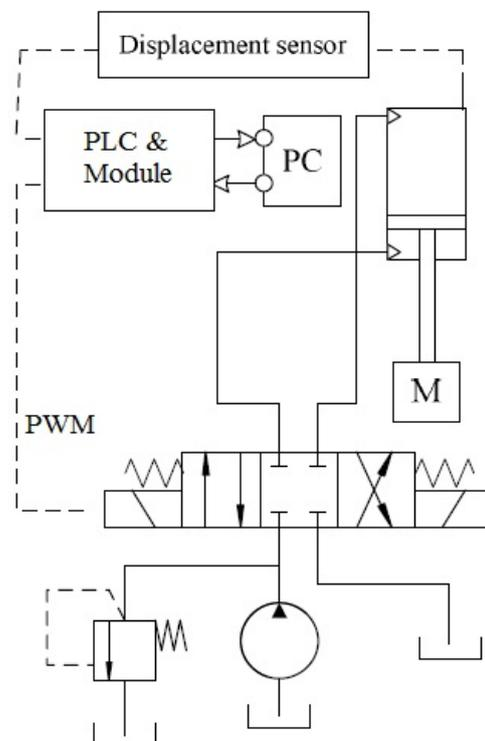
Fig. 1. Hydraulic control circuit
