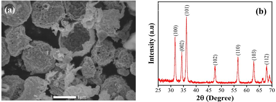
**Fig. 1.** SEM images (a) and XRD pattern (b) of ZnO hollow microspheres.
