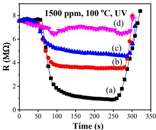
Fig. 6. Response of the M2 sensor film to 1500 ppm a) ethanol, b) NH<sub>3</sub>, c) acetone, d) LPG at 100 °C under UV illumination.
