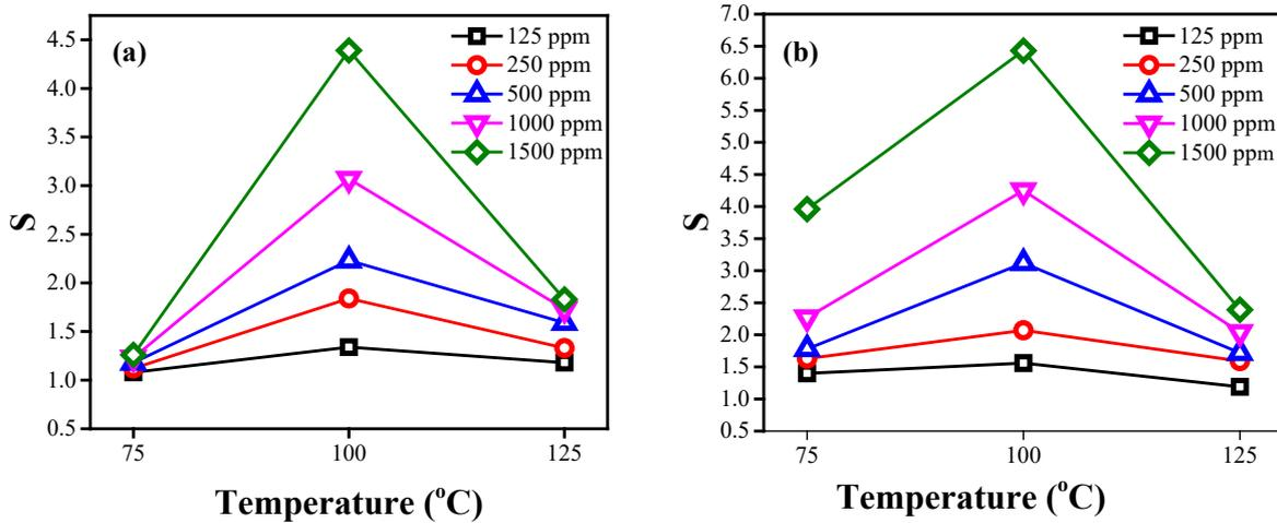
Fig. 5. Sensitivity of M1 (a) and M2 (b) at temperatures range 75-125 °C. All measurements were realized under UV illumination.
