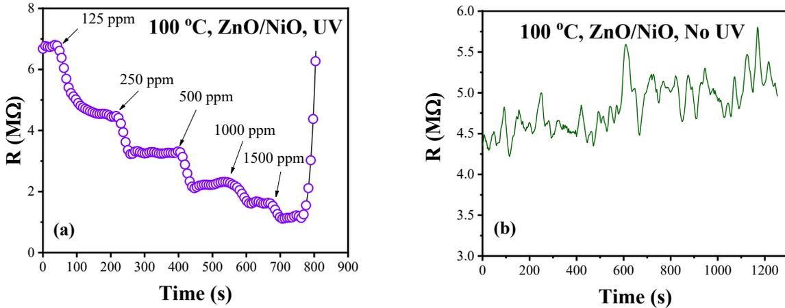
Fig. 4. Transient response of the M2 sensor film to ethanol vapor (125-1500 ppm) at 100 °C under UV illumination (a) and in the dark (b).
