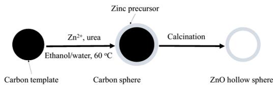
**Fig. 2.** Schematic illustration of the formation of ZnO hollow microspheres.
