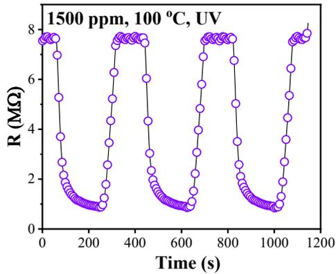
**Fig. 7.** Response of the M2 sensor film to 1500 ppm ethanol after 5 months at 100 °C under UV illumination.
