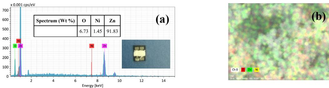
**Fig. 3.** EDX spectrum (a) and elemental mapping (b) of the M2 sensor film.
