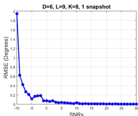
**Fig. 4.** DOA estimation accuracy in AWGN channel with varying SNR
