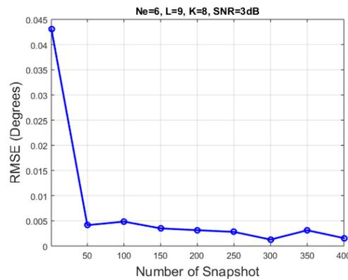
**Fig. 3.** Impact of number of snapshots on DOA estimation accuracy
