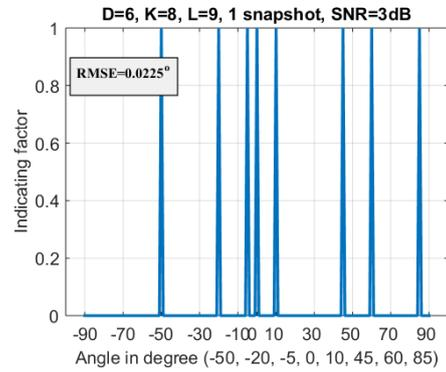
**Fig. 2.** DOA estimation result of eight incoming signals with only one snapshot
