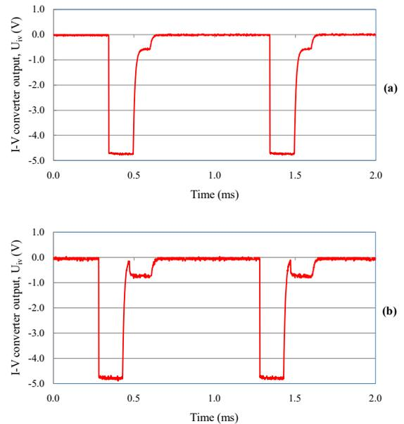
**Fig. 6.** Cross-influence between two pulses of the lights when: (a) there is no idle time, and (b) there is a delay of 80  $\mu$ s
