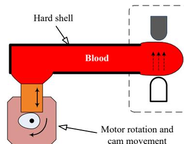
**Fig. 4.** Simple phantom and experimental setup
