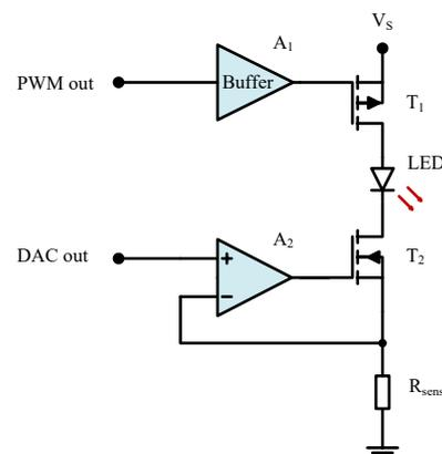
Fig. 2. Simplified schematic of the LED driver
