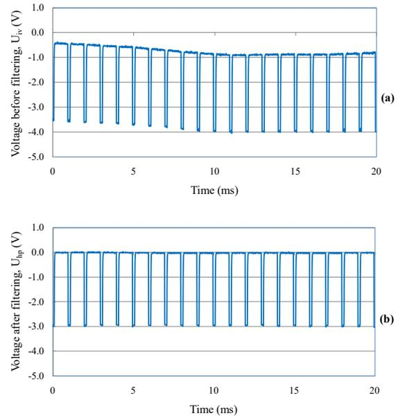
**Fig. 5.** Measured signals when the ambient light is changed: (a) before filtering, and (b) after filtering
