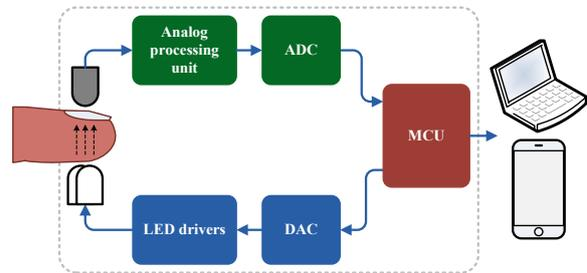
Fig. 1. System hardware with key blocks
