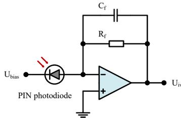
**Fig. 3.** Simplified schematic of the I-V converter
