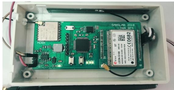
Fig. 4. Main-board of the radioactive sources monitoring device.
