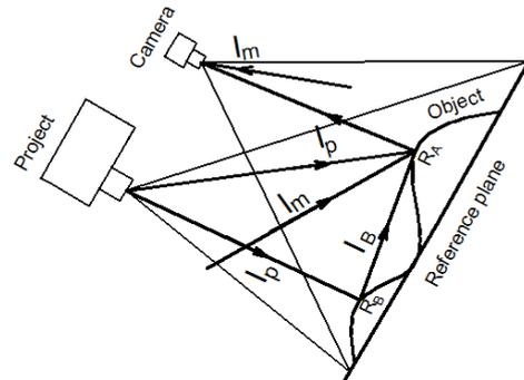
Fig. 1. Principle of surface reflection.
