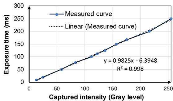
**Fig. 5.** Graph of the between captured intensity and exposure time
