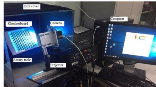
Fig. 3. Setup the experimental system
