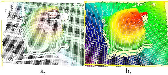
Fig. 8. 3D point cloud of an aluminum mount in single exposure (a), in merged point clouds at 3 appropriate exposures (b),
