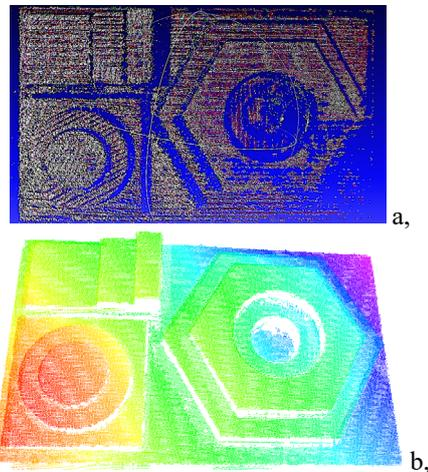
Fig. 10. 3D point cloud of an aluminum part in single exposure (a), in merged point clouds at 3 appropriate exposures (b),
