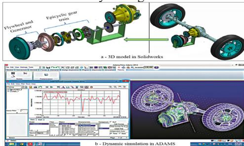
Fig. 6. Experimental model in SolidWorks and ADAMS
