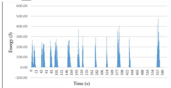
**Fig. 13.** Energy recovered on the NEDC driving cycle
