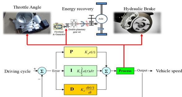
Fig. 3. Block diagram of the simulation
