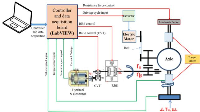
Fig.7. Experimental model diagram
