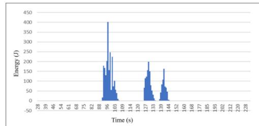
Fig. 11. Energy recovered on the ECE R15 driving cycle
