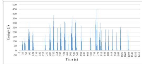
Fig. 10. Energy recovered on the FTP 75 driving cycle
