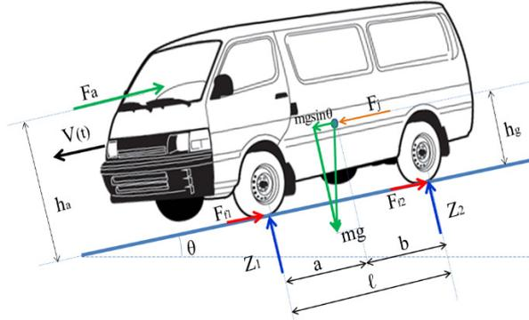
**Fig. 2.** The free-body diagram of the forces acting on the vehicle
