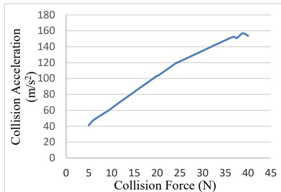
Fig. 8. The relationship of force and acceleration
