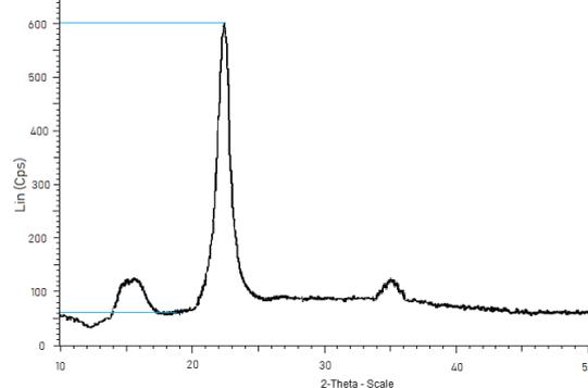
**Fig. 6.** X-ray diffraction patterns of nanocellulose
