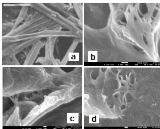
**Fig. 2.** SEM of (a) raw material, (b) 40 mins hydrolysis, (c) 50 mins hydrolysis and (d) 60 mins hydrolysis.
