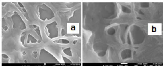
**Fig. 3.** SEM of (a) hydrolysis at 35°C, (b) hydrolysis at 45°C.
