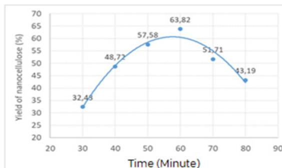
**Fig. 1.** Effect of hydrolysis time on yield of nanocellulose.
