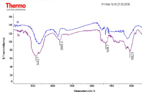
**Fig. 4.** FTIR spectra of (a) bleached *Wood pulp* and (b) nanocellulose.
