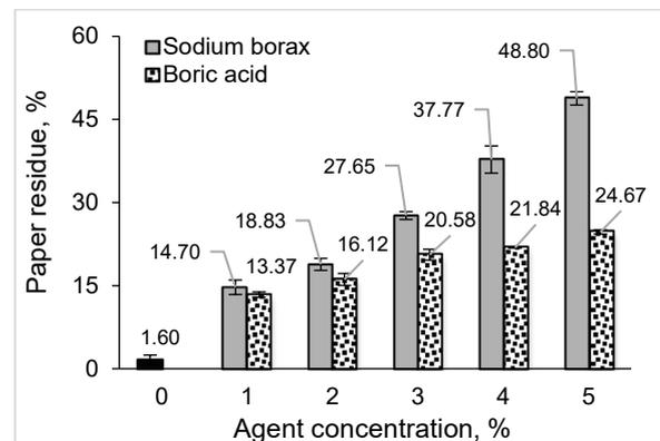
**Fig. 1.** Influence of borax and boric acid concentration on flammability of paper when used separately; impregnation and burning time were 5 min and 30 s, respectively
