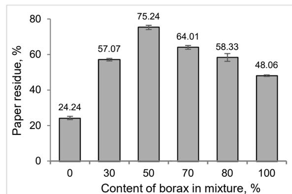
**Fig. 2.** Influence of borax/ boric acid ratio on flammability of paper when used in mixtures; impregnation and burning time were 5 min and 30 s, respectively
