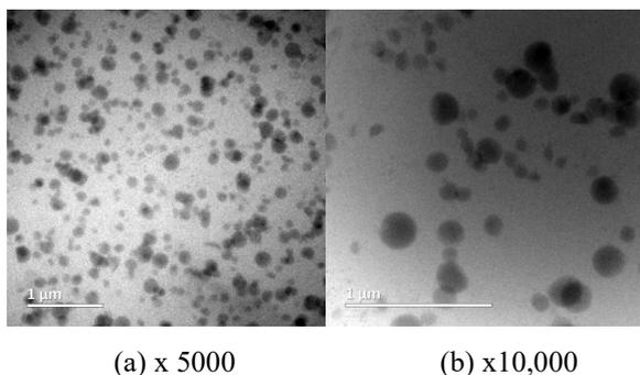
Fig. 4. TEM images of DPNR-g-VTES 0.033-1.5 at two magnifications (a) x5000 and (b) x10,000
