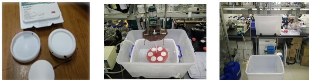
Fig. 1. Chemcatcher sampler, Experiment setup and sampling
